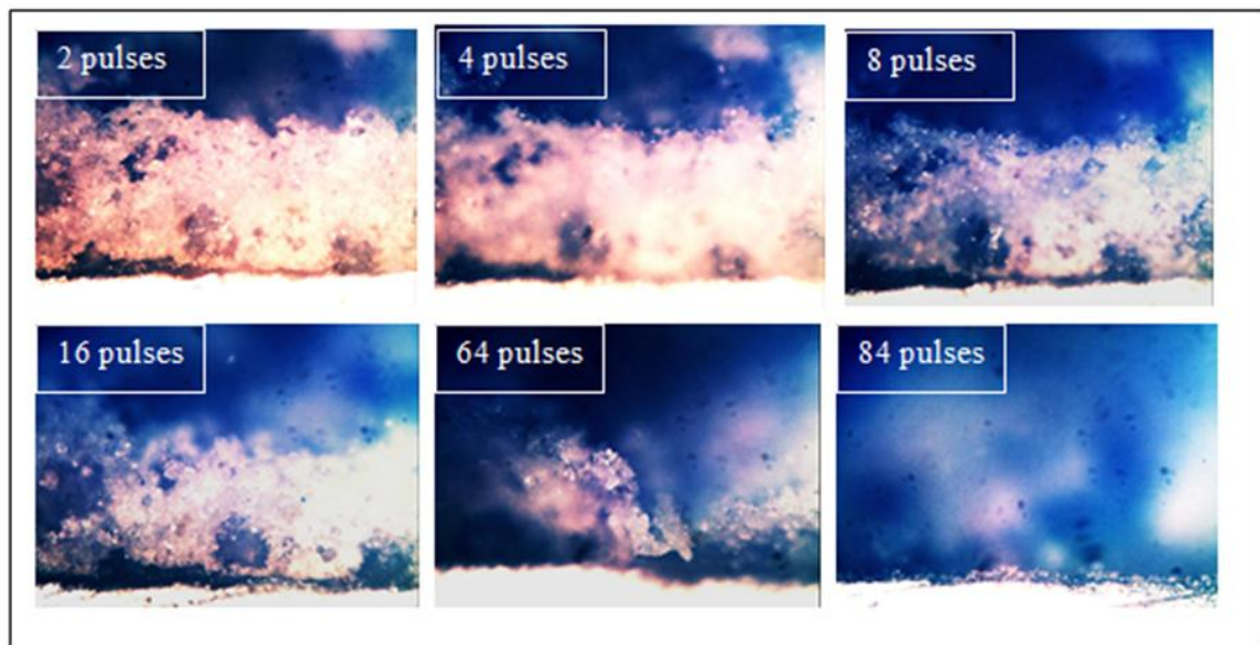
Fig. (1): Microscopic cross section image of iron plate cleaned with different number of Nd: YAG laser pulses and 4.89x10 10 W/cm 2 laser intensity.
