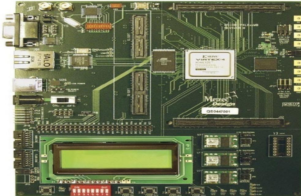
**Figure (7): Virtex-4 System Board [13]**
