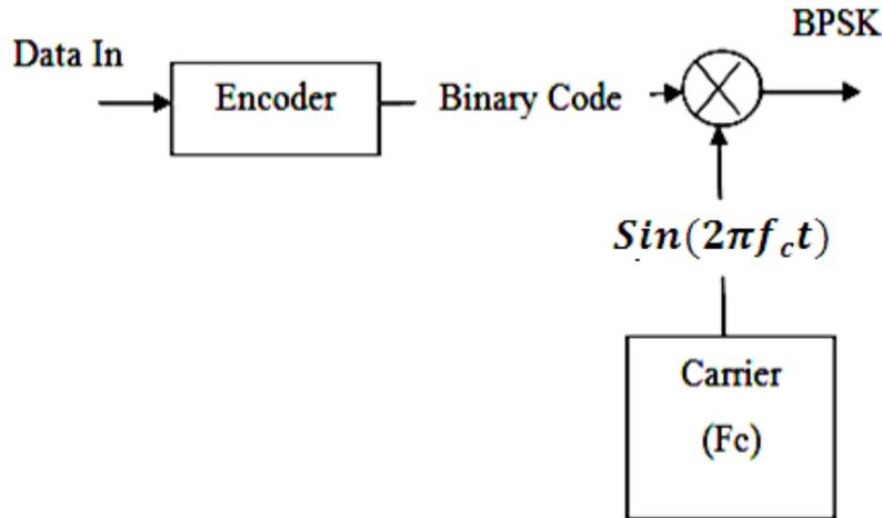
Figure (2): Block diagram of BPSK modulator design
