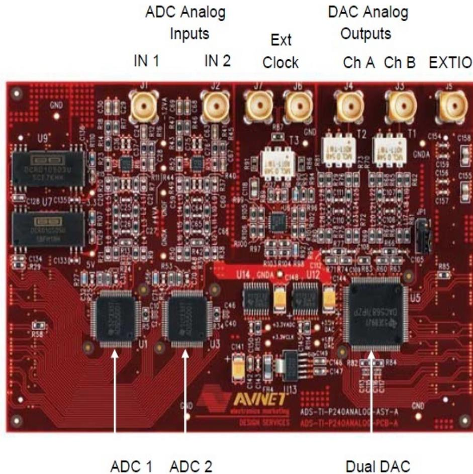
Figure (8): Avnet Electronics Marketing P240 Analog Module [23] .
