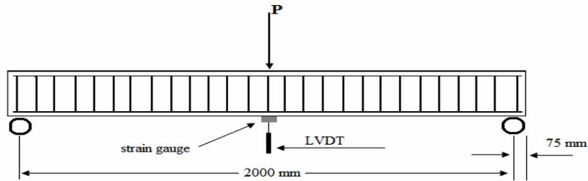
Figure (2): Loading reigns of analyzed beams<sup>[9]</sup>.
