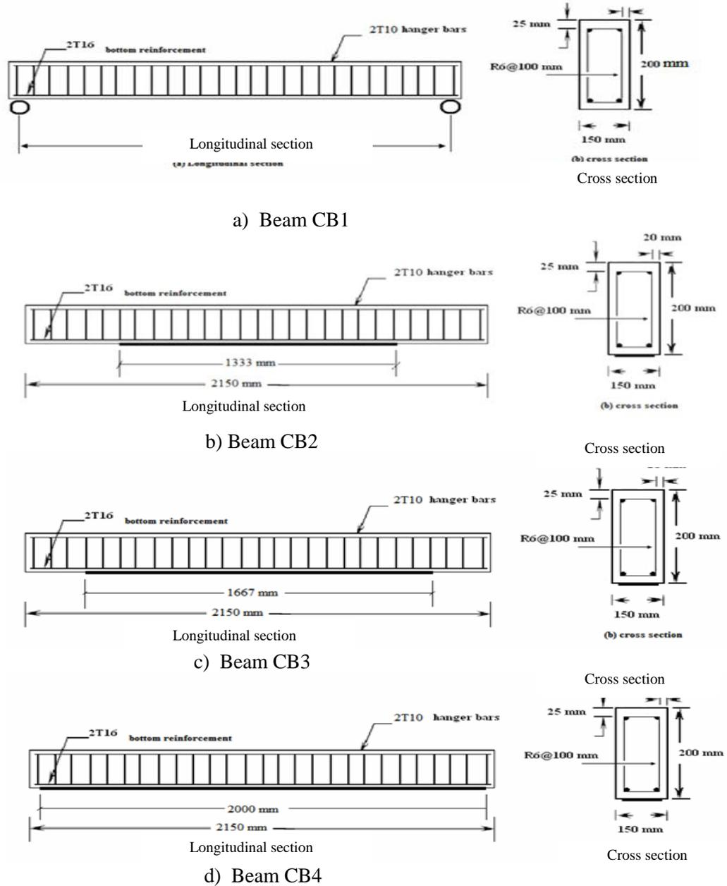
Figure (1): Geometrical properties of analyzed beams<sup>[9]</sup>.
