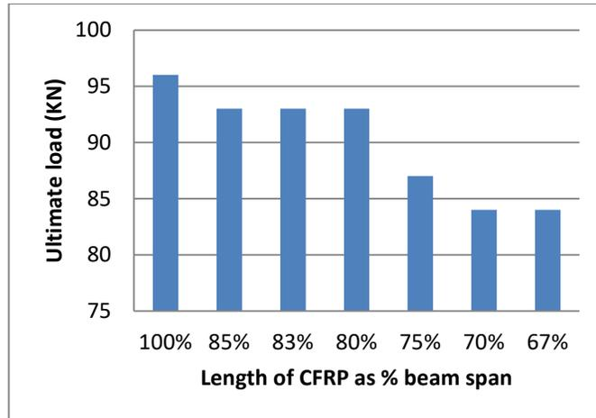
Figure(7) : Comparisons of the ultimate failure loads .
