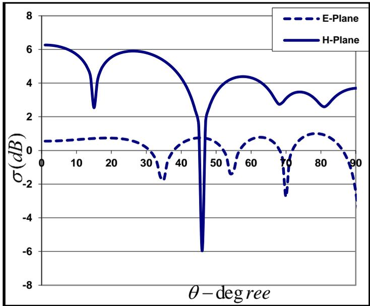
Fig.(7). Computed normalized backscatter cross sections for coated conducting cylinder (thickness of dielectric( $d$ )=0.1cm,)
