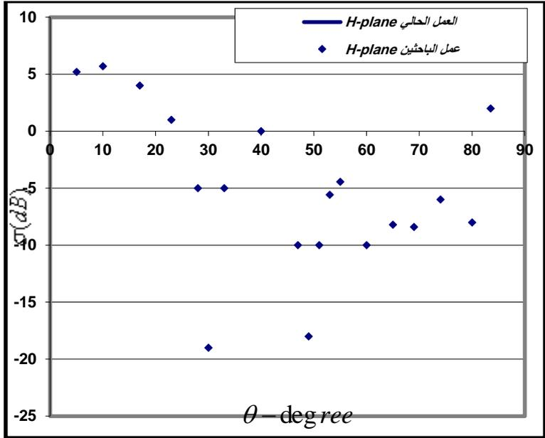
Figure (6): Computed normalized backscatter cross sections for cylinder( $d=0, Z=0$ ) .a-  $\phi\phi$  polarization. b-  $\theta\theta$  polarization.
