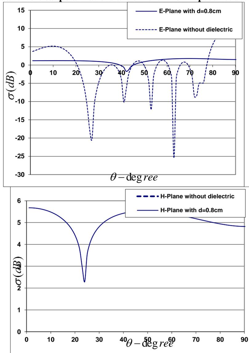
Fig.(10): RCS Comparing for the conducting cylinder and the conducting cylinder with dielectric coating.
