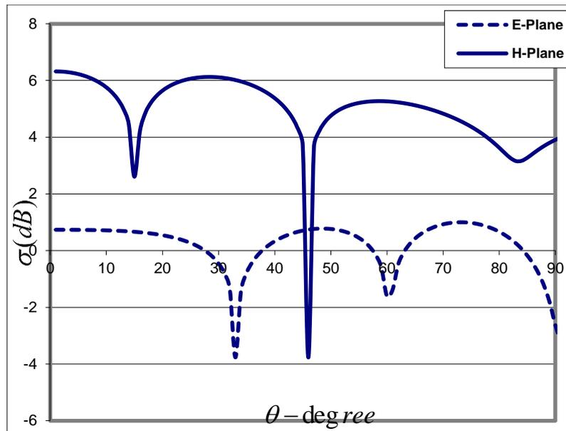
Fig.(8). Computed normalized backscatter cross sections for coated conducting cylinder (thickness of dielectric(d)=0.4cm,)
