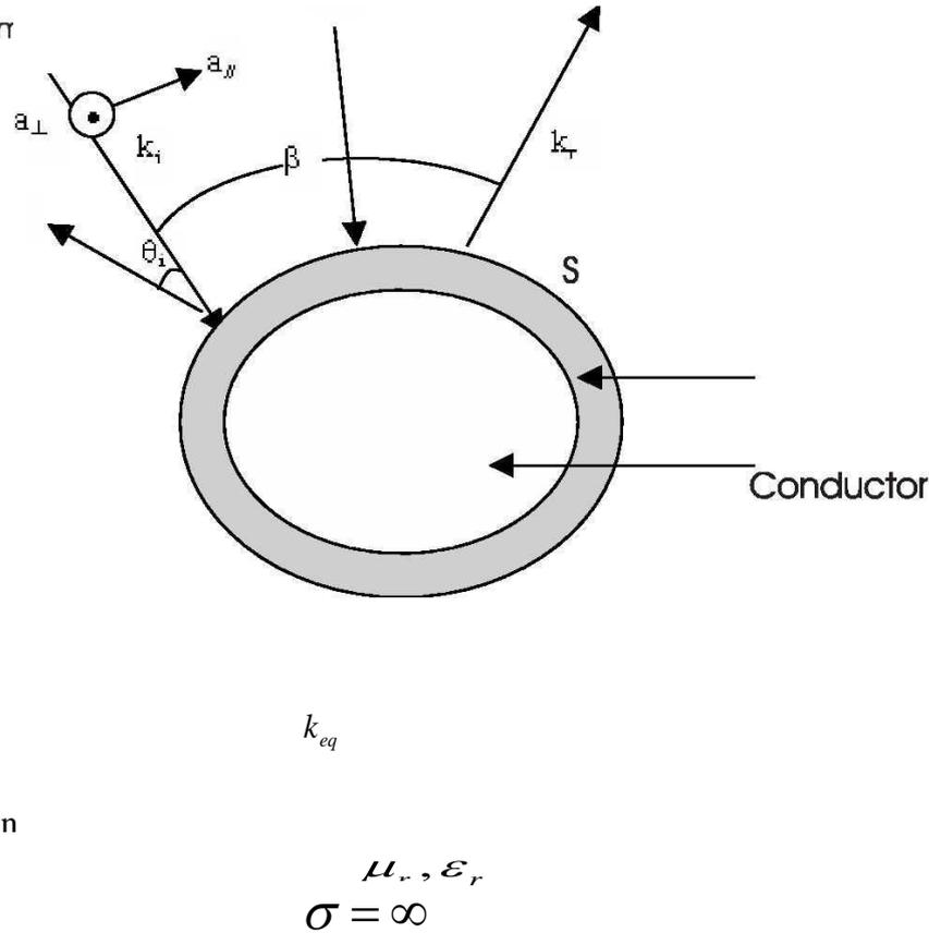
**Figure (1): Bistatic scattering from a coated object.**
