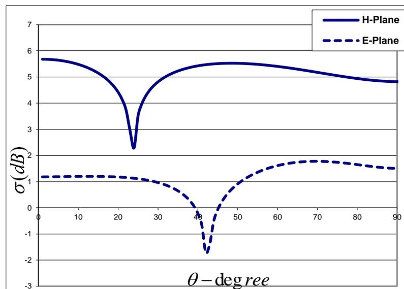
Fig.(9). Computed normalized backscatter cross sections for coated conducting cylinder (thickness of dielectric(d)=0.8cm) .
