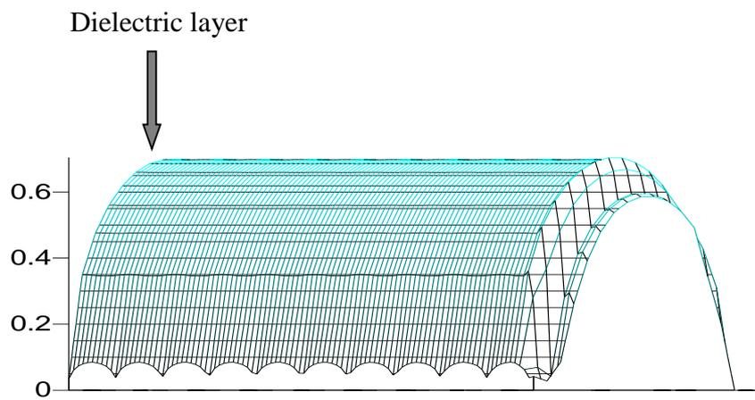
**Figure (5): Distribution of meshes for Cylinder with dielectric layer by MOM.**
