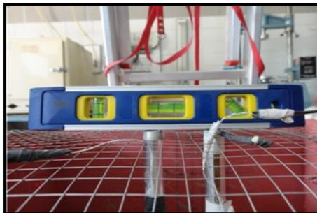
Plate (5): Placing of piles in the soil tank.
