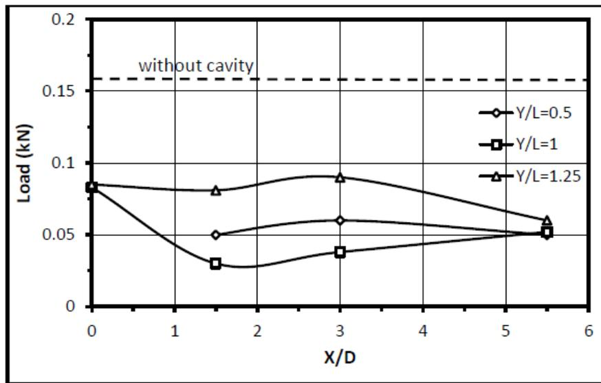
**Figure (10): Variation of load of pile group (1x2) versus cavity location of ( $X/D$ ) at different depths of cavity with ( $d/D=1$ ).**
