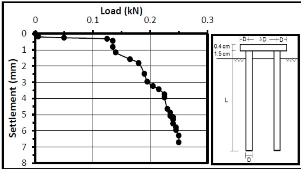
Figure (8): Load-Settlement curve of group piles (1x2) embedded in soil without cavity, L=20 cm, D=1.6 cm.
