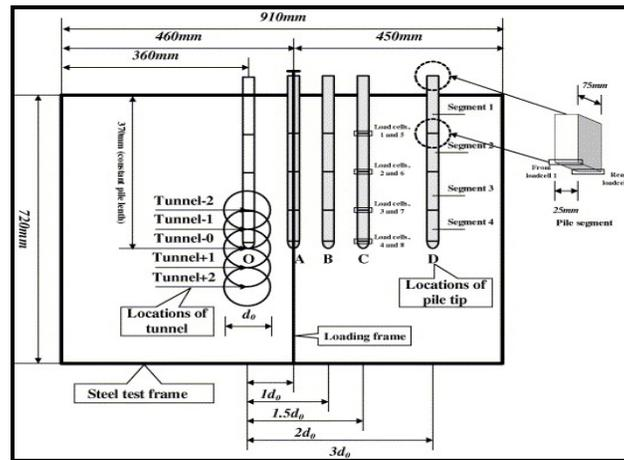
Figure (3): Schematic diagram for the pile–soil–tunneling interaction model test (after Lee and Bassett, 2007).
