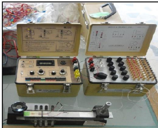
Plate (3): Calibration of the strain indicator.
