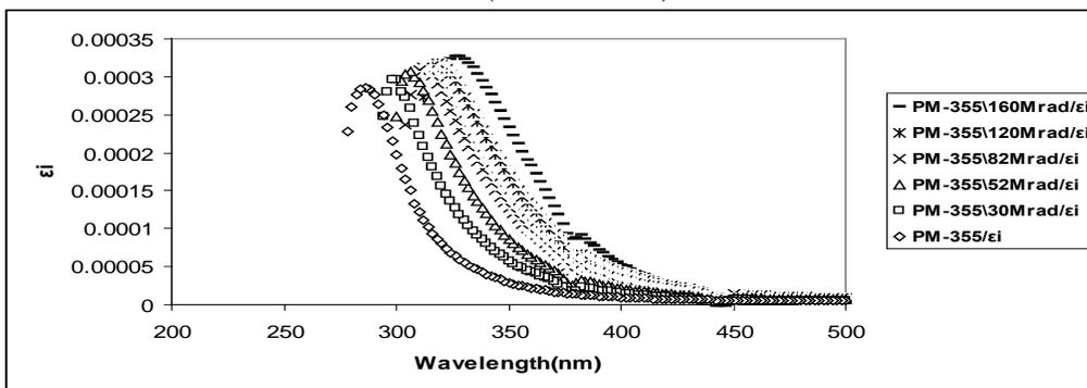
Figure.(14): The variation of imaginary part of the dielectric constant versus wavelength for the PM-355 before and after irradiation with  $\gamma$ -ray dose within range of(30-160Mrad).
