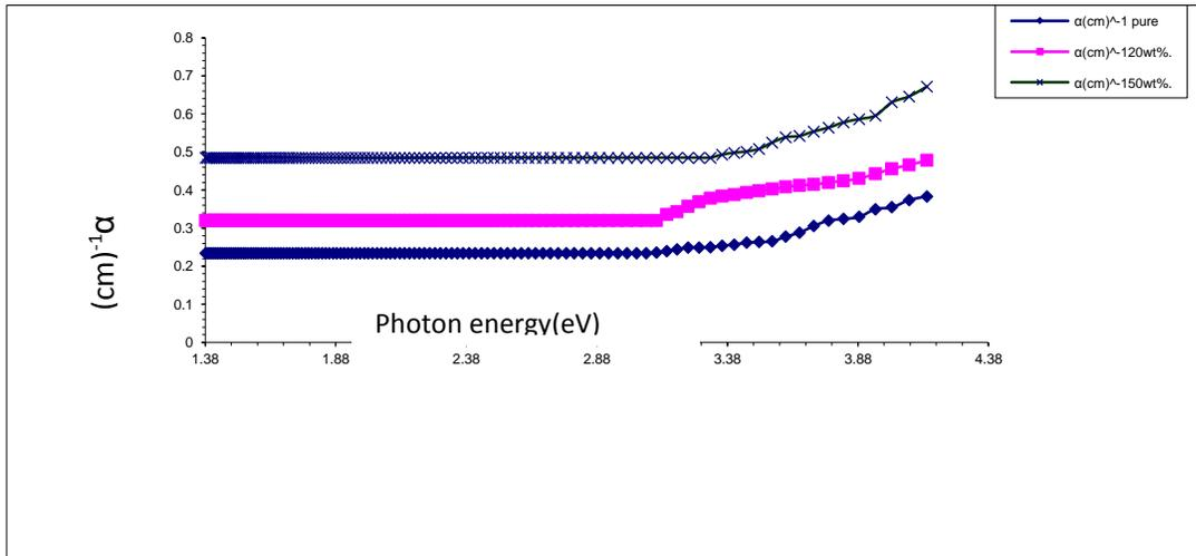
**Figure (1) The relationship between the absorption coefficient and photon energy of the PVA-Ni composites**
