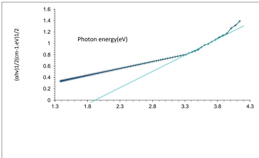
**Figure (4) the relationship between  $(\alpha h\nu)^{1/2}(\text{cm}^{-1}.\text{eV})^{1/2}$  and photon energy of PVA-Ni composites for 50wt.% Ni**
