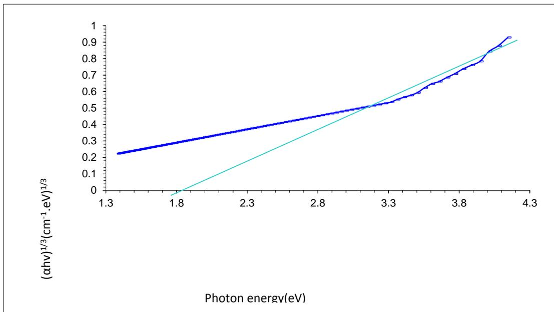
**Figure (7) the relationship between  $(\alpha h\nu)^{1/3}(\text{cm}^{-1}.\text{eV})^{1/3}$  and photon energy of of PVA-Ni composites for 50wt.% Ni**
