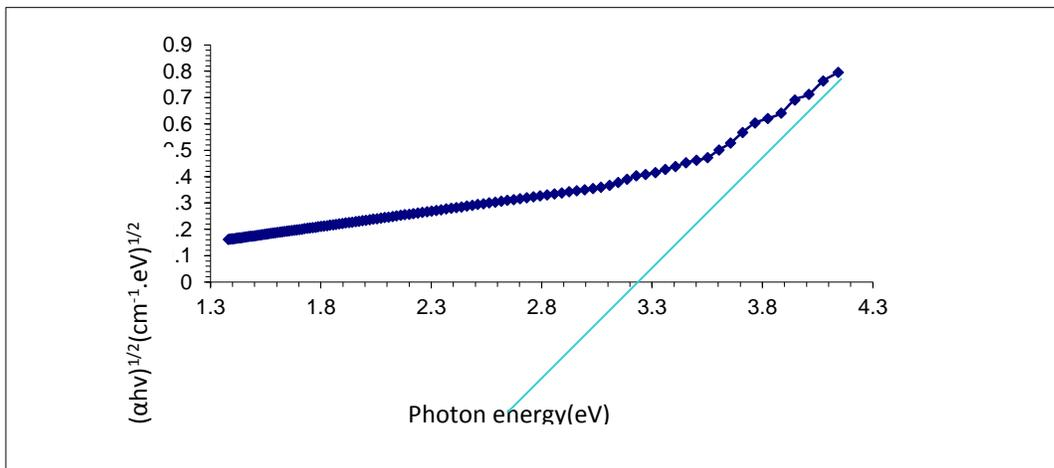
**Figure (2) the relationship between  $(\alpha h\nu)^{1/2} (\text{cm}^{-1} \cdot \text{eV})^{1/2}$  and photon energy of pure polymer (PVA).**
