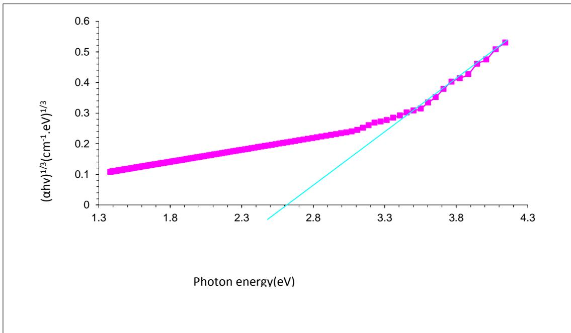
**Figure (5) the relationship between  $(\alpha h\nu)^{1/3} (\text{cm}^{-1} \cdot \text{eV})^{1/3}$  and photon energy of pure polymer (PVA).**
