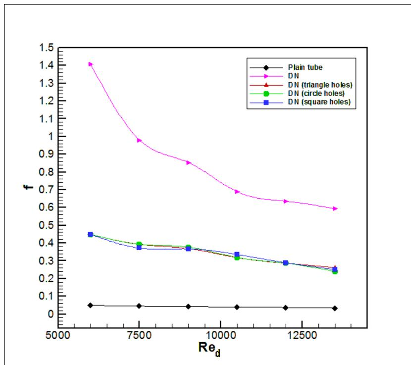
Figure.(9) Friction factor vs. Reynolds number
