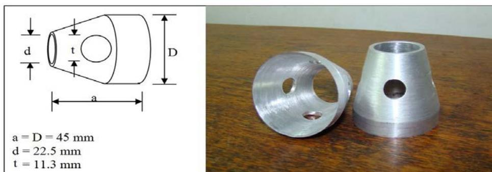
Figure. (3) Circle shape perforation Nozzle-turbulators
