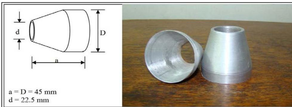
Figure. (2) Dimensions of the nozzle-turbulators.
