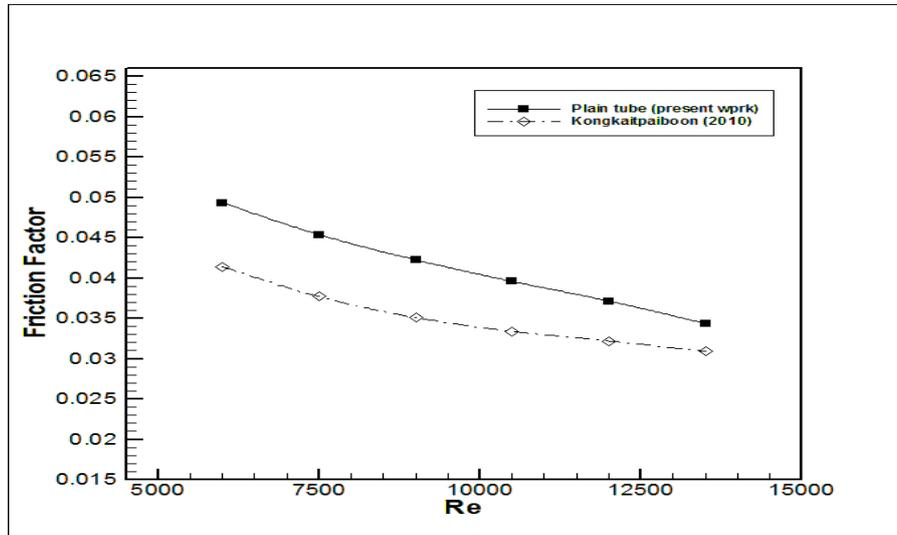
Figure.(7) Verification of Friction factor of plain tube
