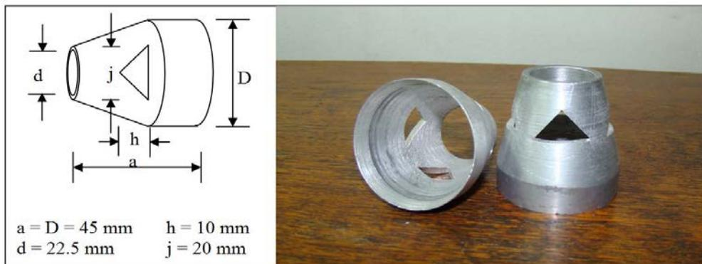
Figure. (5) Triangle shape perforation Nozzle-turbulators
