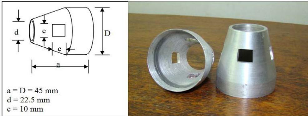
Figure. (4) Square shape perforation Nozzle-turbulators
