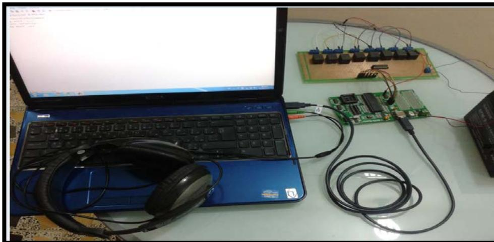
Figure (5): Interface between Laptop and Wheelchair.
