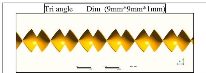
Figure 2. Twisted tape tri-angle shape
