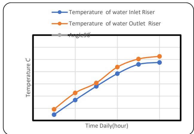
**Figure 17.** Temperature of water inlet & outlet riser at (16<sup>th</sup> of August)
