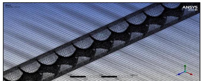
Figure 7. Tetrahedral mesh in a tube and twisted tape
