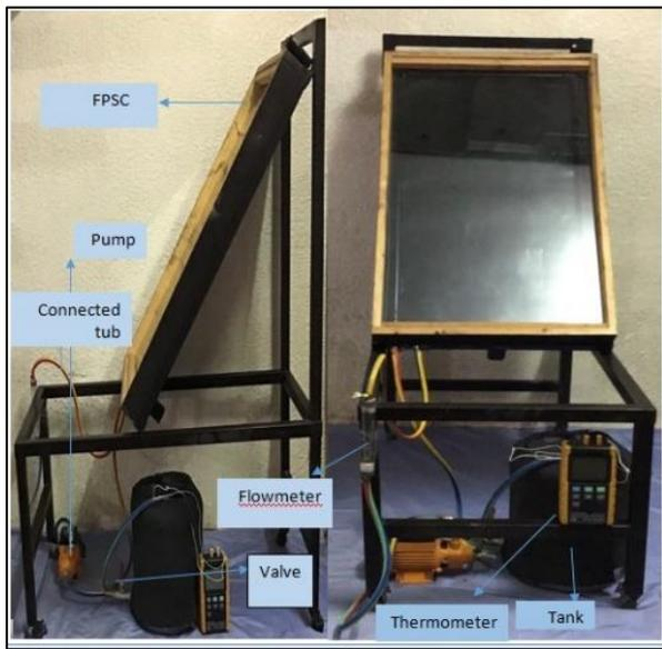
**Figure 13.** Photo Flat plat solar collector under examination
