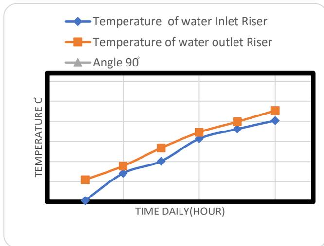
**Figure 14.** Temperature of water inlet & outlet riser at (13<sup>th</sup> of August)
