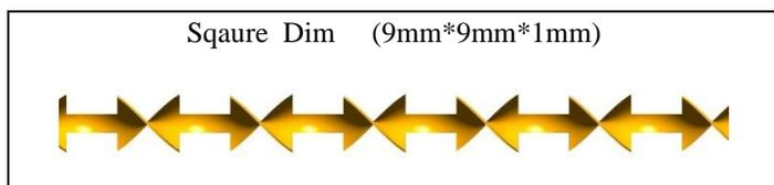
Figure 3. Twisted tape as square shape (3pitch)
