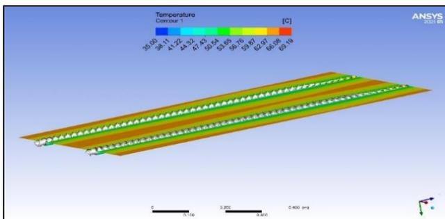
**Figure 34.** Temperature of water twisted tape at Numerical study
