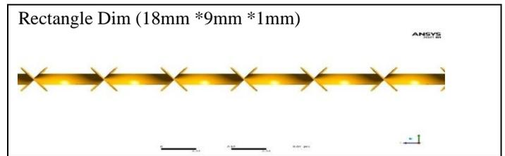
Figure 4. Twisted tape rectangle shape
