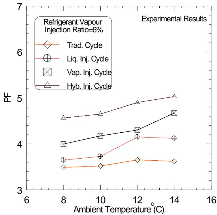
Figure (12) Effect of ambient temperatures on PF.
