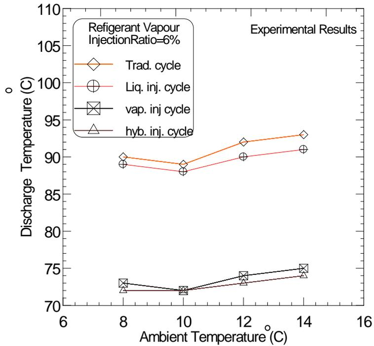
Figure (7) Effect of ambient temperatures on compressor discharge temperature.
