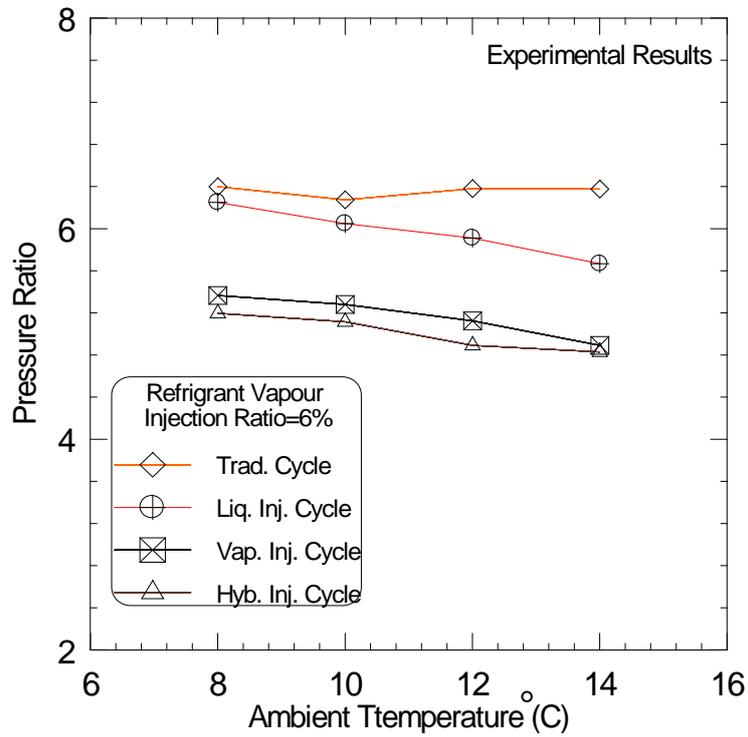
Figure (5) Effect of ambient temperatures on pressure ratio.
