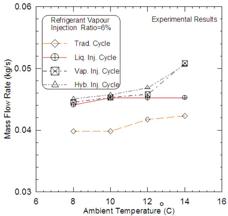
Figure (8) Effect of ambient temperatures on mass flow rate.
