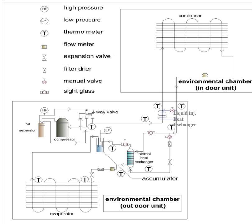
Figure (3) Experimental heat pump system.
