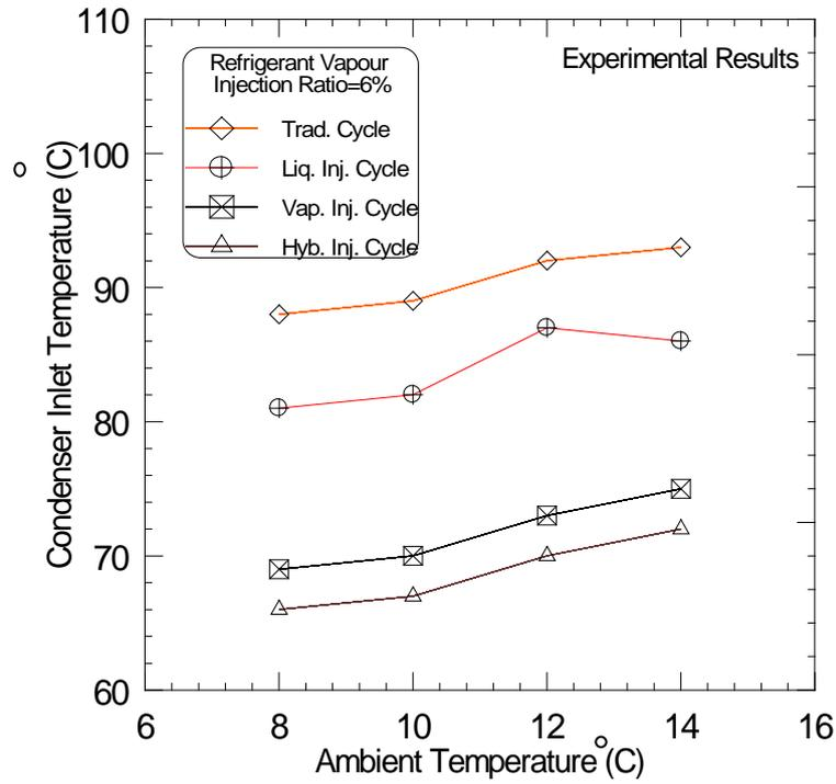
Figure (9) Effect of ambient temperatures on condenser inlet temperature.
