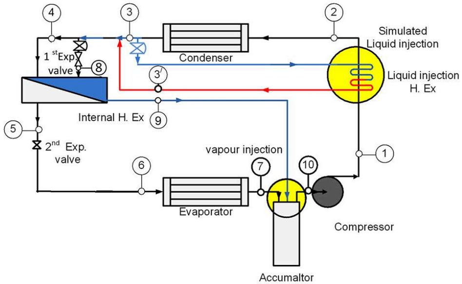
Figure (1) Schematic diagram of hybrid injection cycle.
