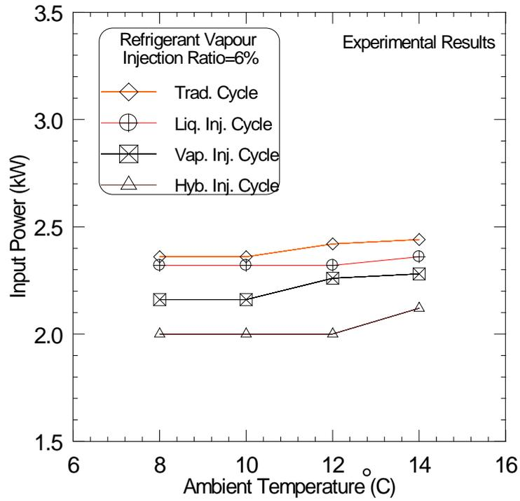
Figure (11) Effect of ambient temperatures on input power.
