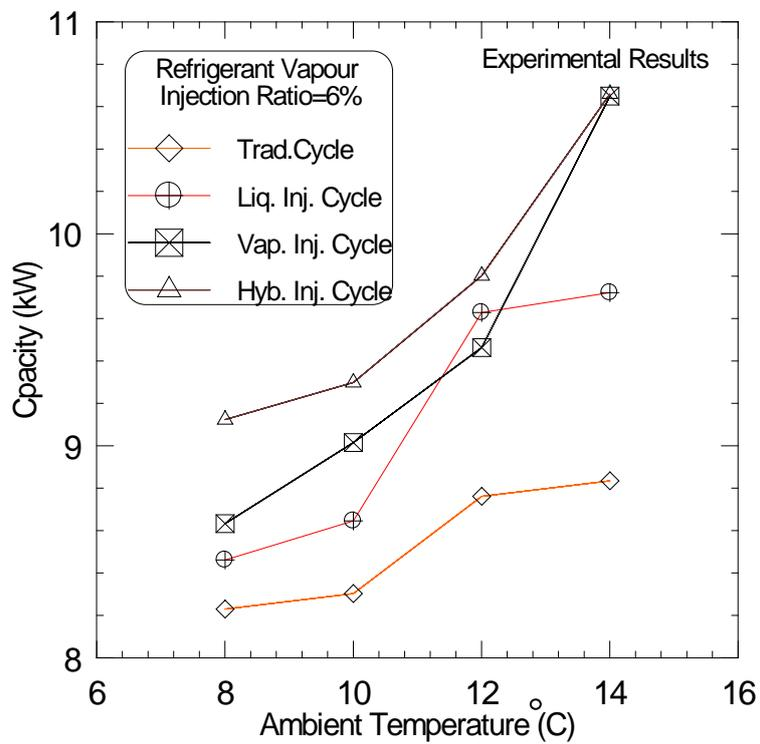
Figure (4) Effect of ambient temperatures on heating capacity.
