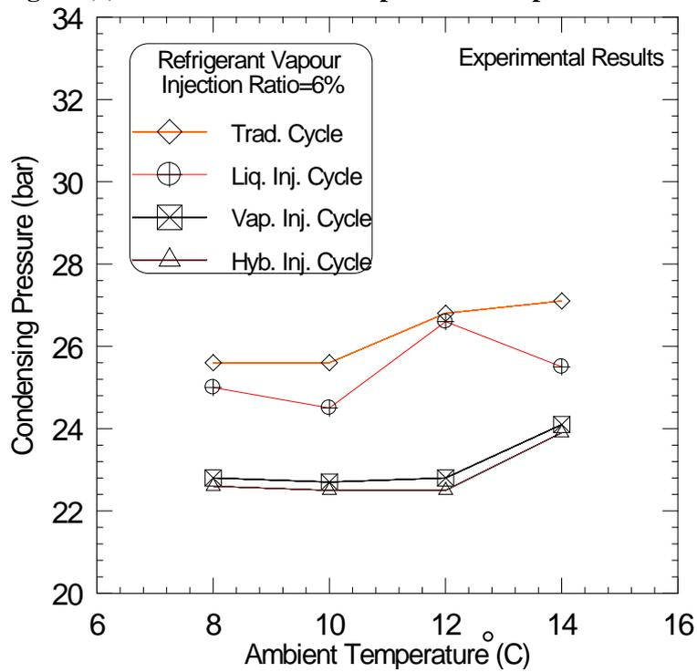
Figure (6) Effect of ambient temperatures on condensing pressure.
