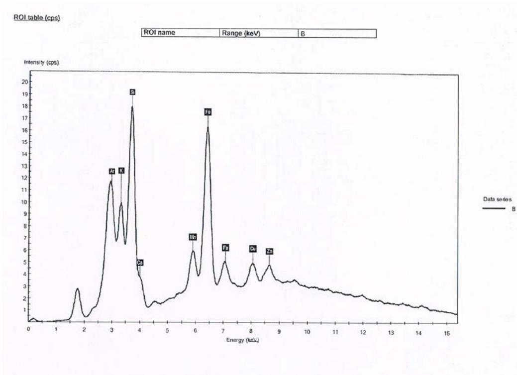
Figure (1):- (XRF) test for rice husk burned at 900°C.
