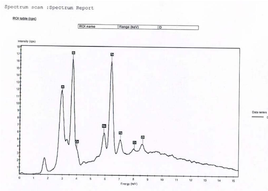
Figure (3): (XRF) test for rice husk burned at 1300°C.
