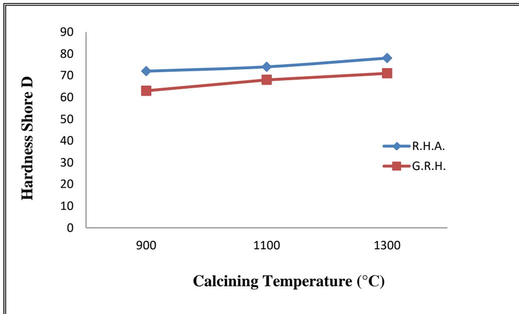
Figure (10):-The relation between hardness and Calcining temperatures.
