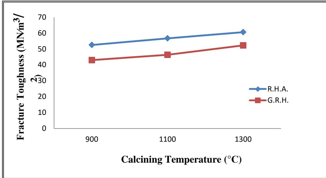
Figure (9):-The relation between impact fracture toughness and Calcining temperatures.
