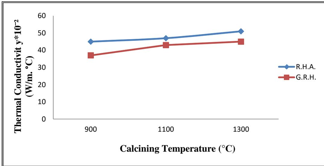
Figure(11):-The relation between thermal conductivity and Calcining temperatures.
