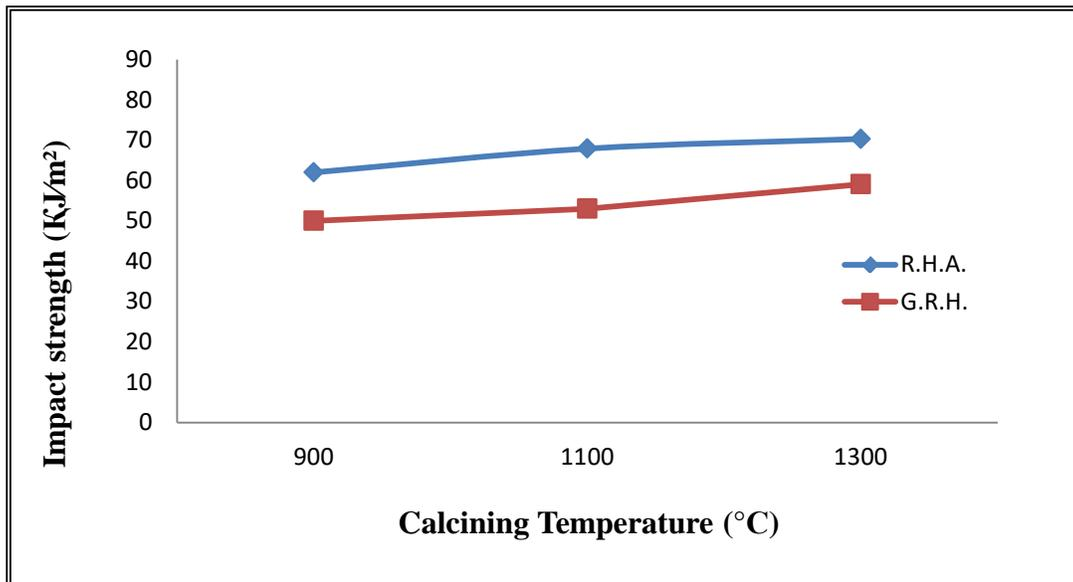
Figure (8):-The relation between impact strength and Calcining temperatures.
