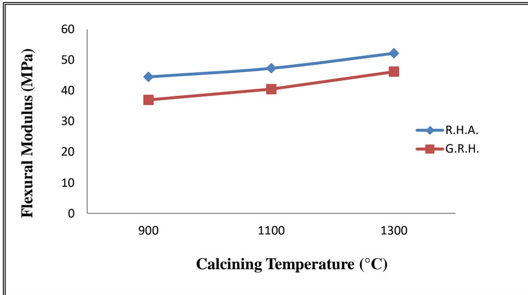
Figure (7):The relation between flexural modulus(  $E_{bend}$  ) and Calcining temperatures.
