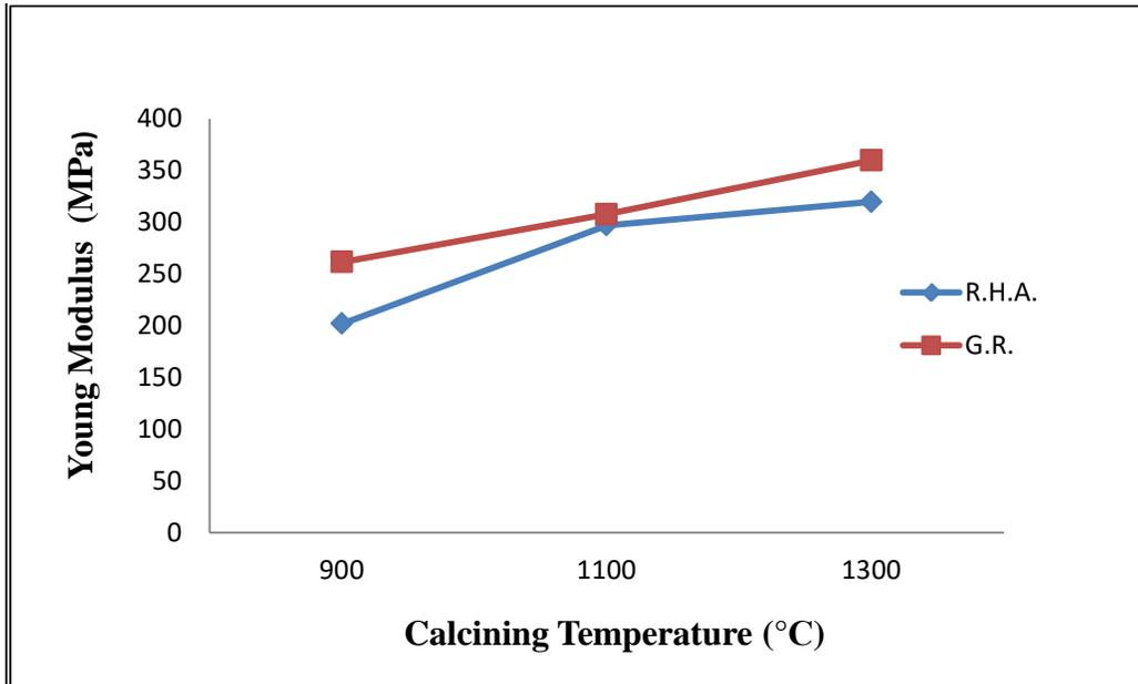
Figure (5):The relation between young modulus of elasticity and calcining temperatures.
