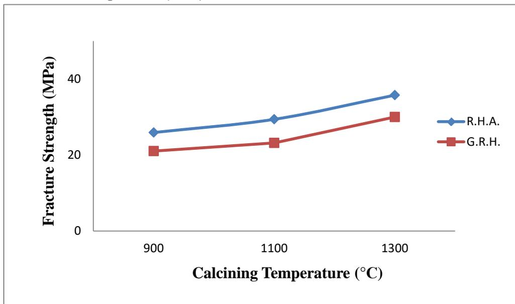
Figure (4): The relation between stress at fracture point and calcining temperatures.
