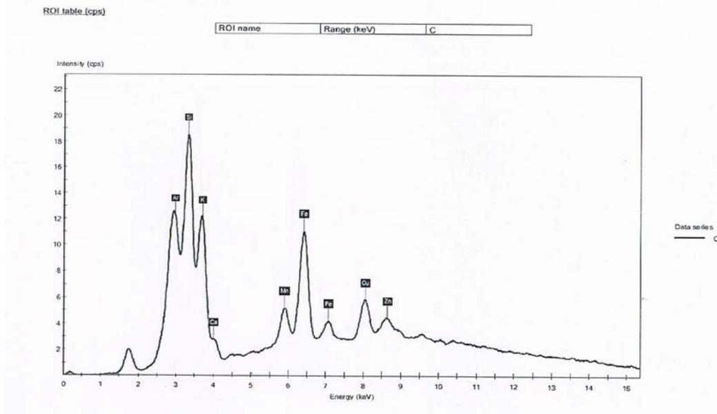
Figure (2): (XRF) test for rice husk burned at 1100°C.
