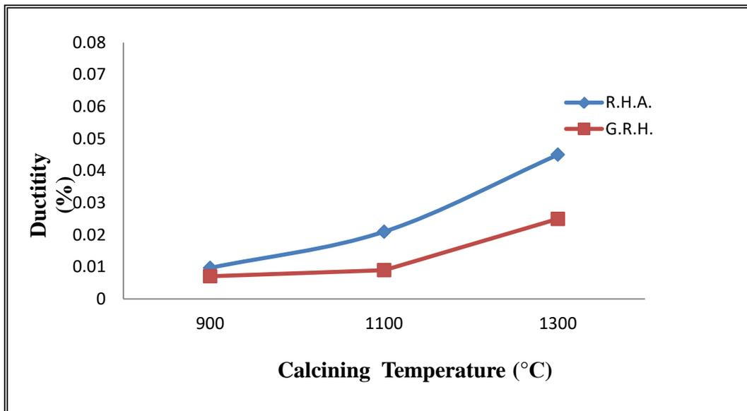
Figure (6):The relation between ductility and calcining temperatures.
