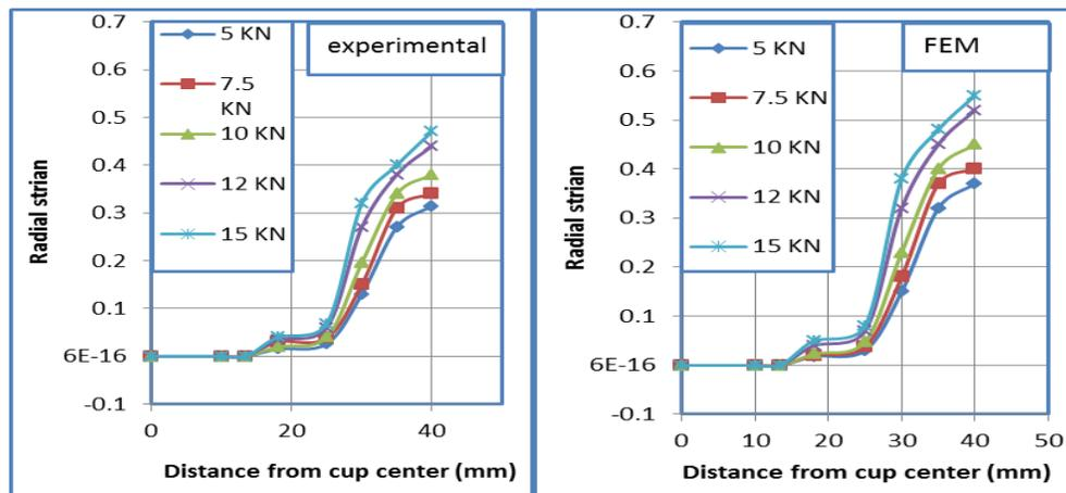
Figure (7) Effect of blank holder force on radial strain
