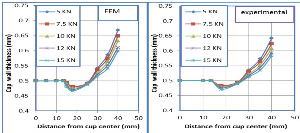
Figure (6) Effect of blank holder force on thickness distribution
