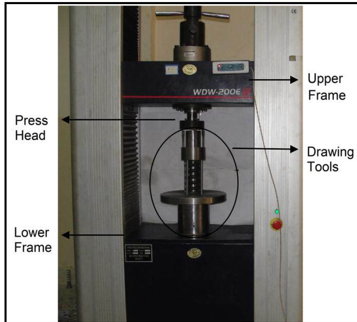
Figure (3) The assembly picture of tools and apparatus used
