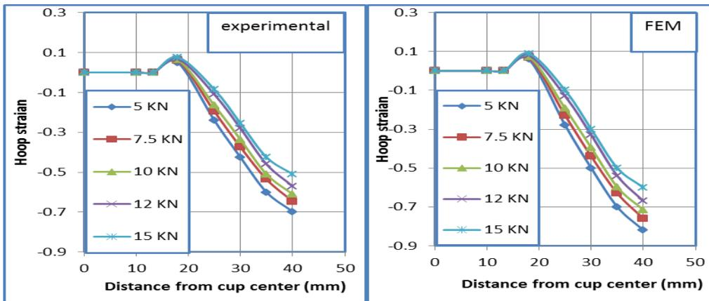
Figure (9) Effect of blank holder force on hoop strain
