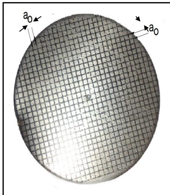
Figure (4) Blank with grid, by using screen printing
