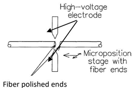
**Figure (1) : Fusion splicing technique.**
