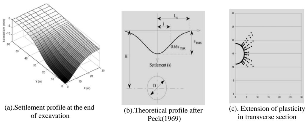
**Figure (3):Free field analysis soil movement and plasticity(after Mroueh,2003)**
