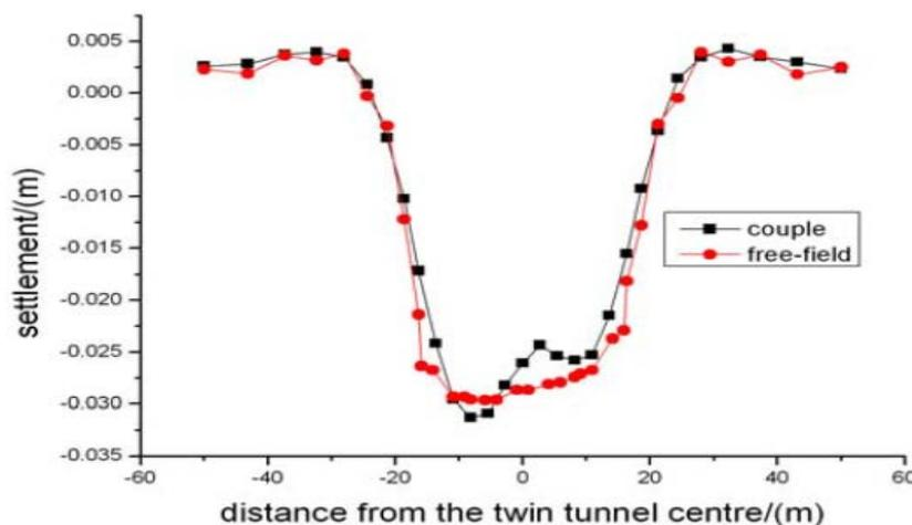
Figure (4): Settlement during twin tunnel excavation (after Ma Keshuan et.al., 2008).
