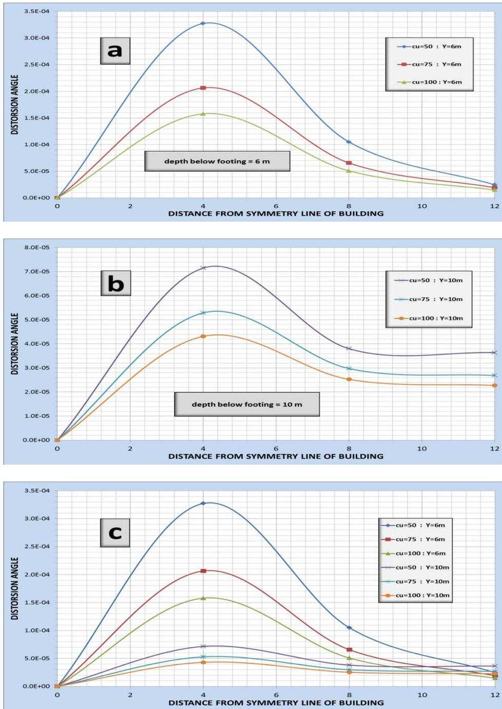
Figure (13) Variation OF Distorsion Angle for different soil types & depth and location of tunnel
