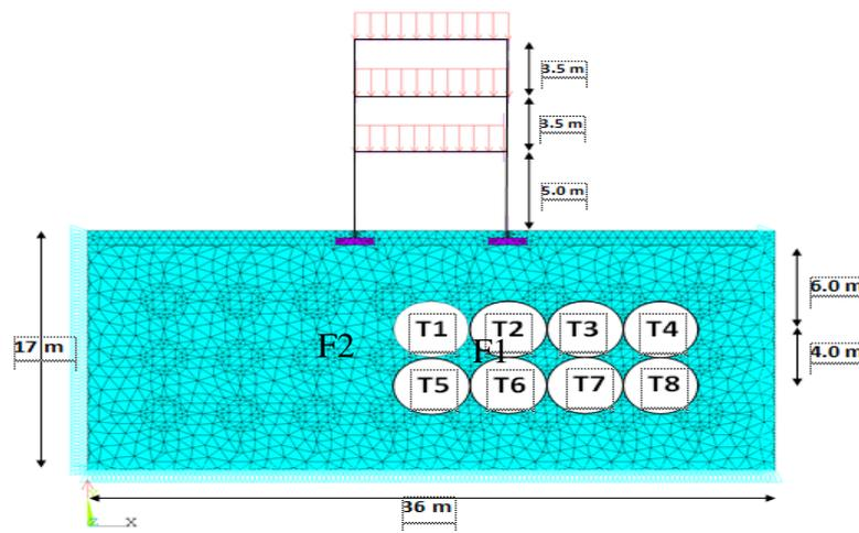
Figure (5) Element formation and study case with tunnel excavated at proposed eight locations below the super-structure
