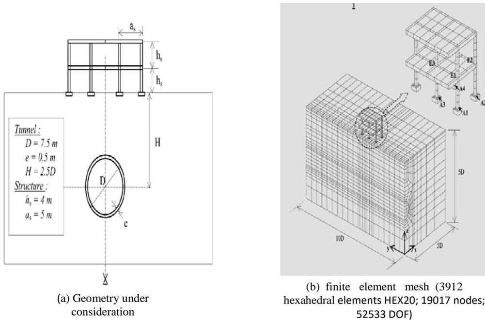
**Figure (2): Full 3-D coupled analysis: presentation of the example (After Mroueh and Shahrour, 2003)**
