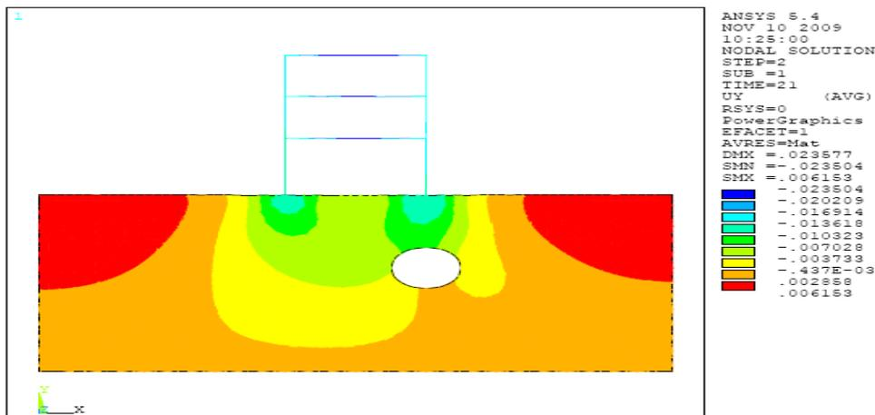
Figure (8) vertical deformation contours for Tunnel depth = 6m
