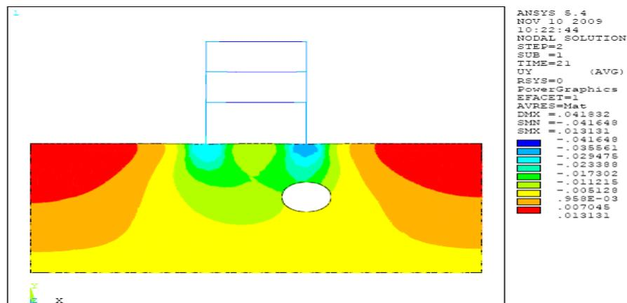
**Figure (6) vertical deformation contours for tunnel depth = 6m
