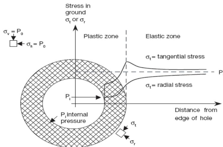
Figure.(1): "Arching" of stresses around a hole in stressed plate (Thomas,2009).
