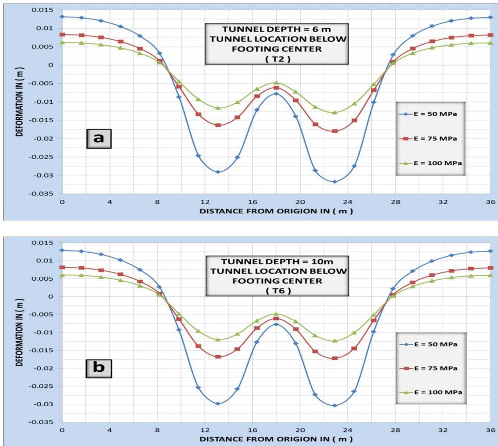
Figure (12) uy variation for critical location of tunnel
