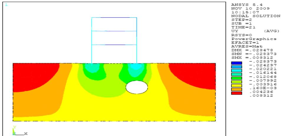
Figure (7) vertical deformation contours for Tunnel depth = 6m
