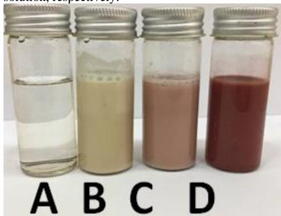
**Figure 1:** Color changes during biosynthesis of selenium nanoparticles (SeNPs) using yeast solution (B) mixed
