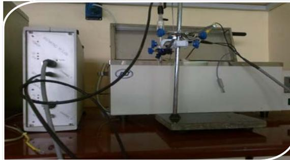
**Figure (2) : Potentiostat for electrochemical corrosion measurement**
