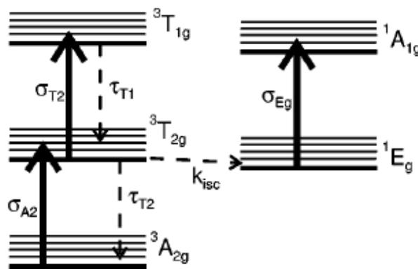
Fig. (1) : Energy levels diagram of  $Cr^{+4} : YAG$  crystal
