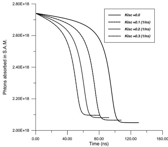
**Fig. (5) : The total photons absorbed in S.A.M. as a function of intersystem crossing ( $K_{isc}$ ).**
