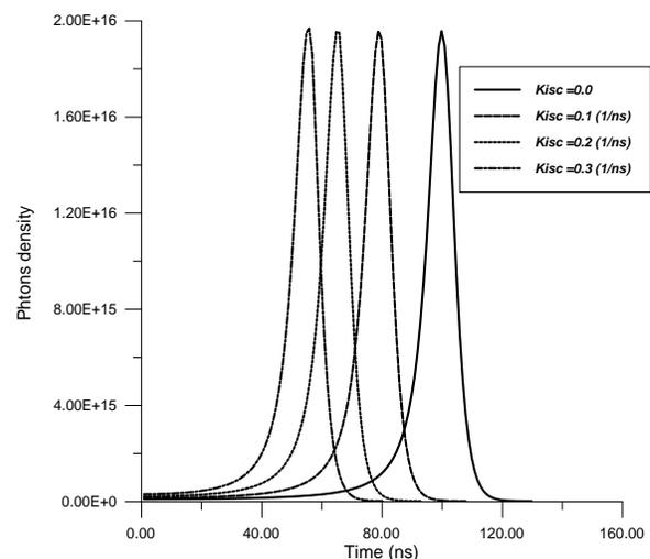
Fig.(3): The profiles of giant pulse related to deferent  $K_{isc}$  values.
