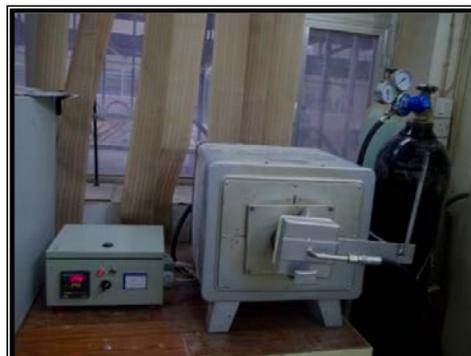
Figure (2) Furnace used for sintering with argon gas.
