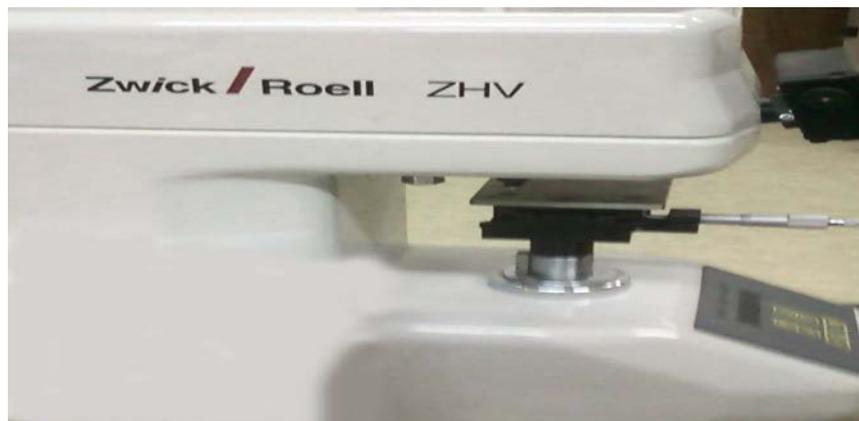
**Figure (5) Hardness Measurement Device
