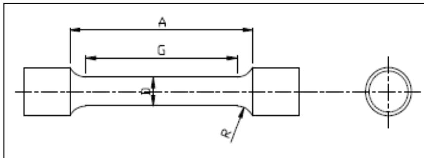
**G: gage length (30mm) , D: diameter (6mm) , R:radius of fillet (6mm) , A: gauge length (36mm)
