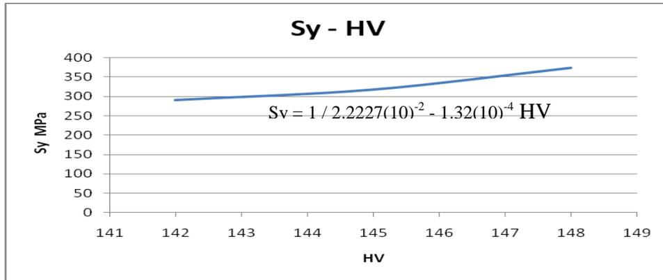
Figure (7) Sy – HV curve
