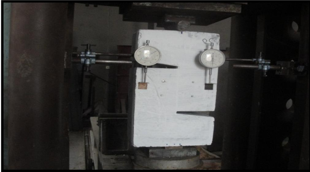
Figure. (2) The test set up the push-off specimens
