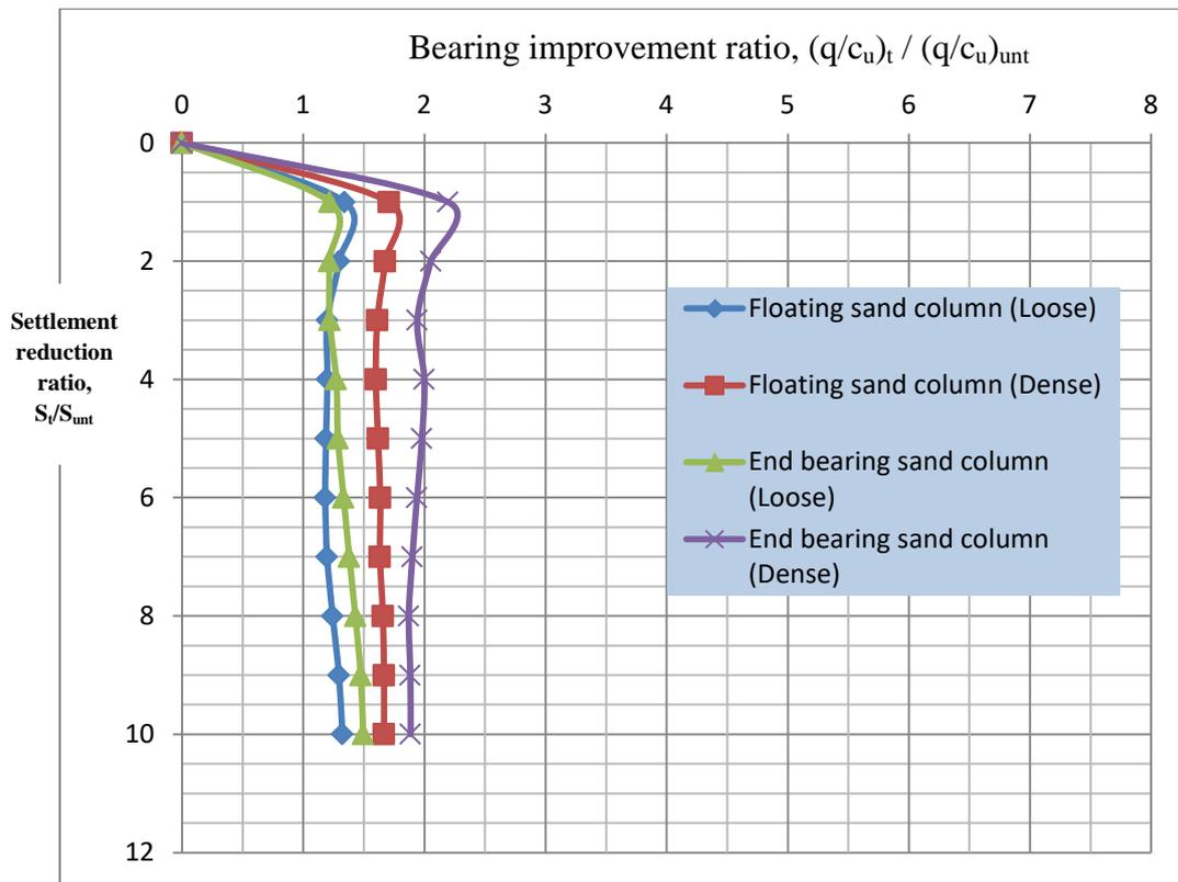
Figure (9): Bearing improvement ratio versus settlement ratio for soil treated with floating sand columns and end bearing sand columns.
