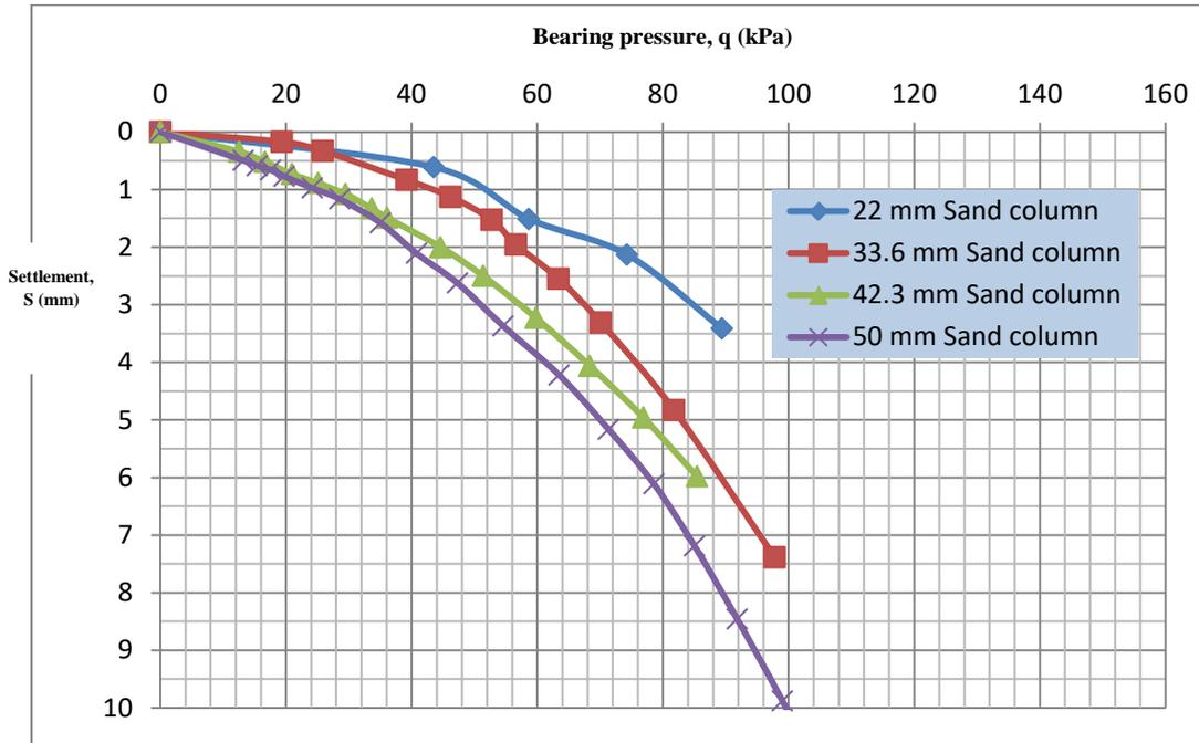
Figure (4): Bearing pressure versus settlement for soil treated with floating sand columns at loose relative density ( $\gamma=17 \text{ kN/m}^3$ ) with different diameters.
