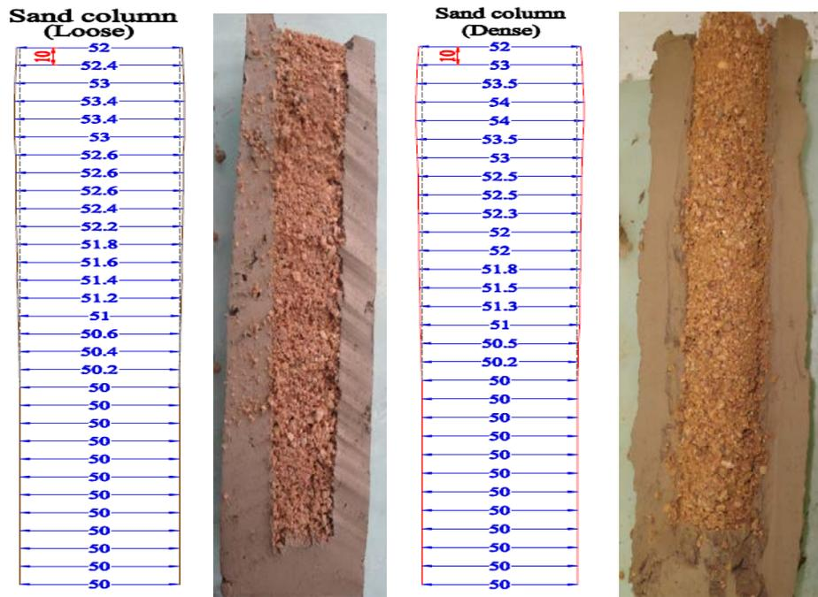
Figure (7): The deformation of floating sand columns at the end of test (all dimensions in mm).
