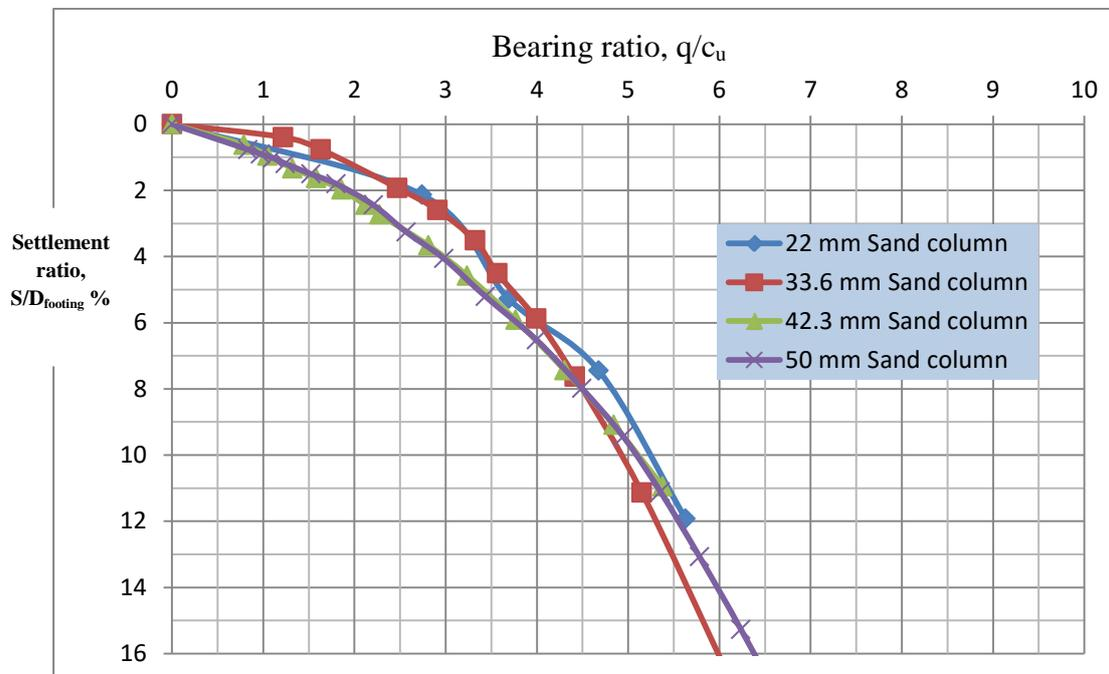
Figure (5): Bearing ratio versus settlement ratio for soil treated with floating sand columns at loose relative density ( $\gamma=17 \text{ kN/m}^3$ ) with different diameters.
