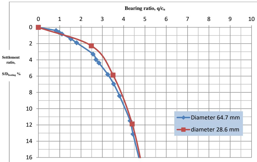
Figure (3): Bearing ratio versus settlement ratio for untreated soil with different footing diameters.
