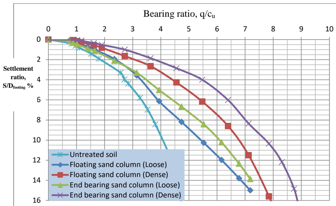
Figure (6): Bearing ratio versus settlement ratio for soil treated with floating sand columns and end bearing sand columns.
