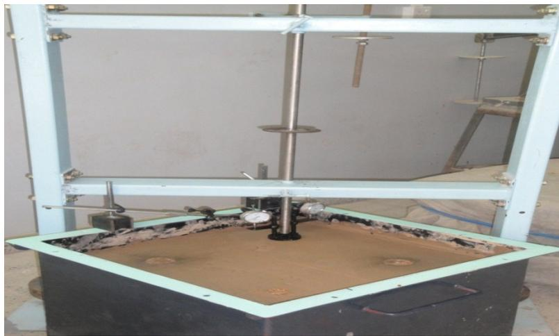
Figure (1):The frame of loading and the steel container
