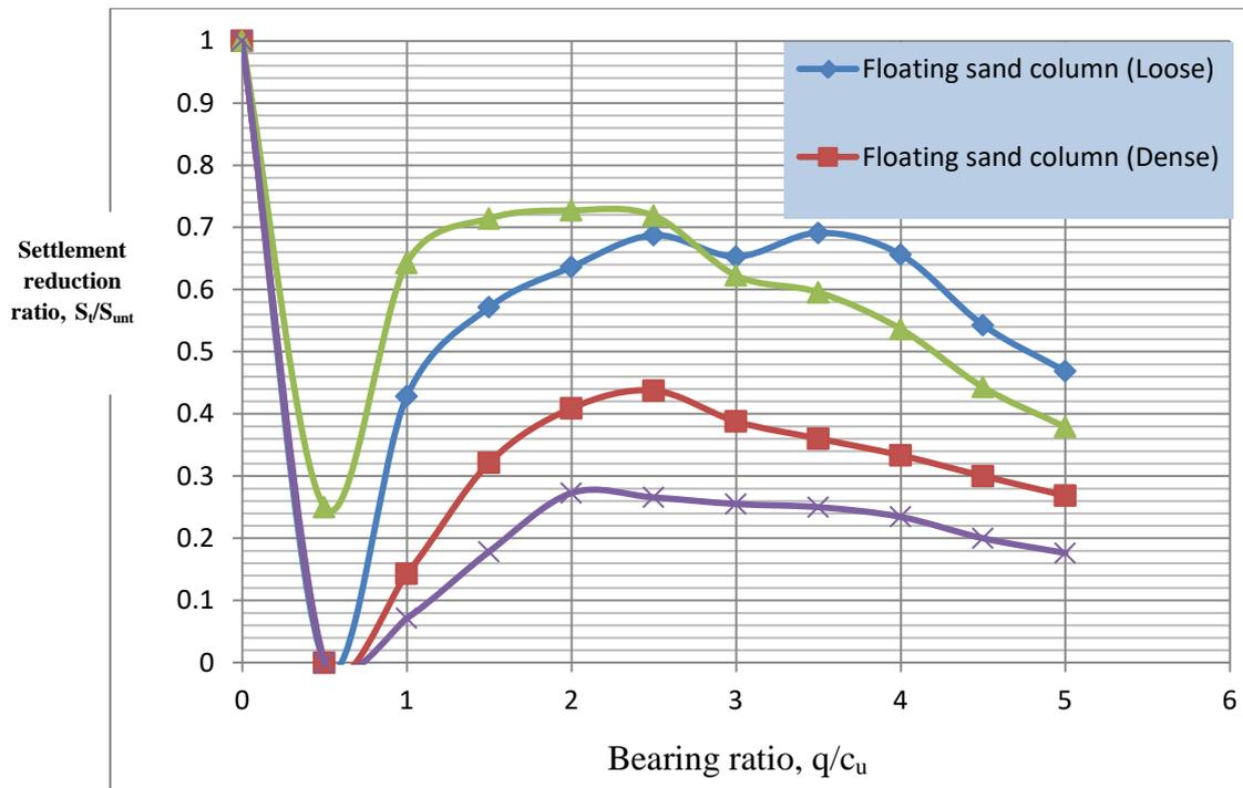
Figure (10):Settlement reduction ratio versus bearing ratio for soil treated with floating sand columns and end bearing sand columns.
