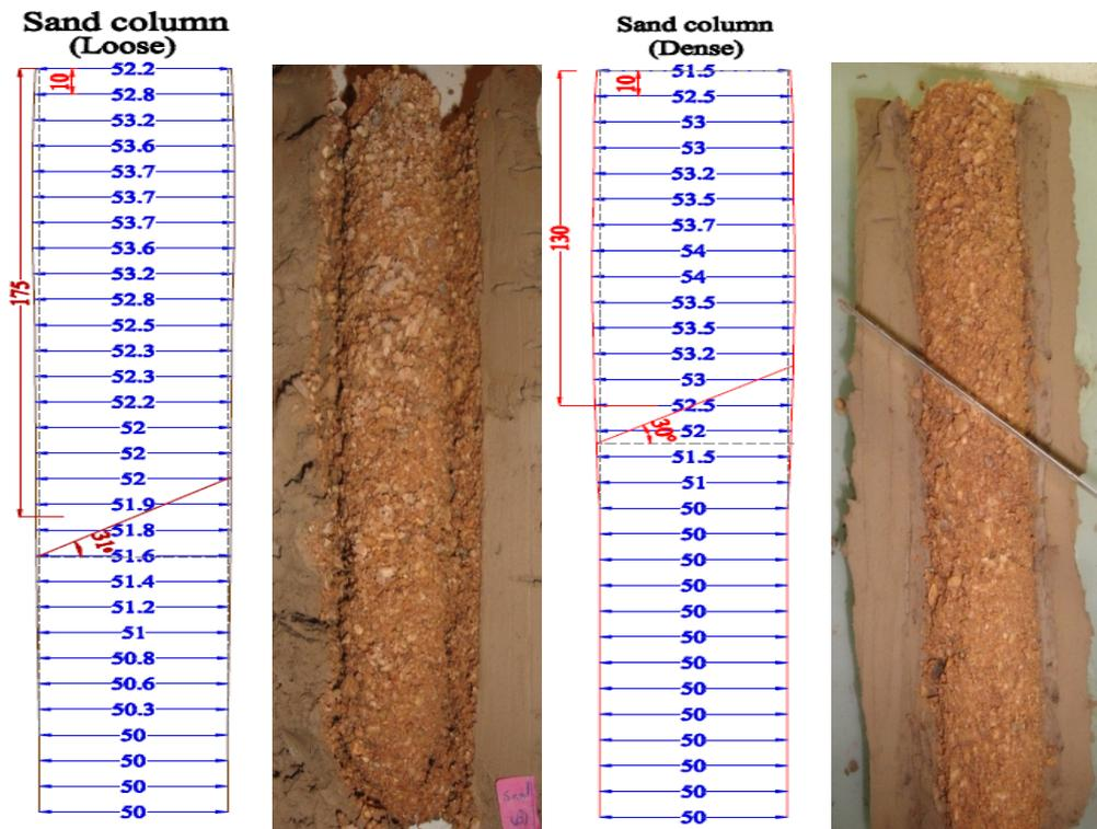
Figure (8): The deformation of end bearing sand columns at the end of test (all dimensions in mm).
