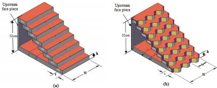
Figure(5) Detail drawing show pieces comprise physical model (a) Traditional shape (b) Labyrinth shape
