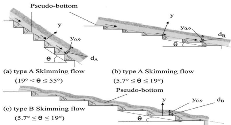
Figure (1) Different faces of skimming flow over stepped spillway ( after Ohtsu Y.Yasuda and M. Takahashi , 2004)
