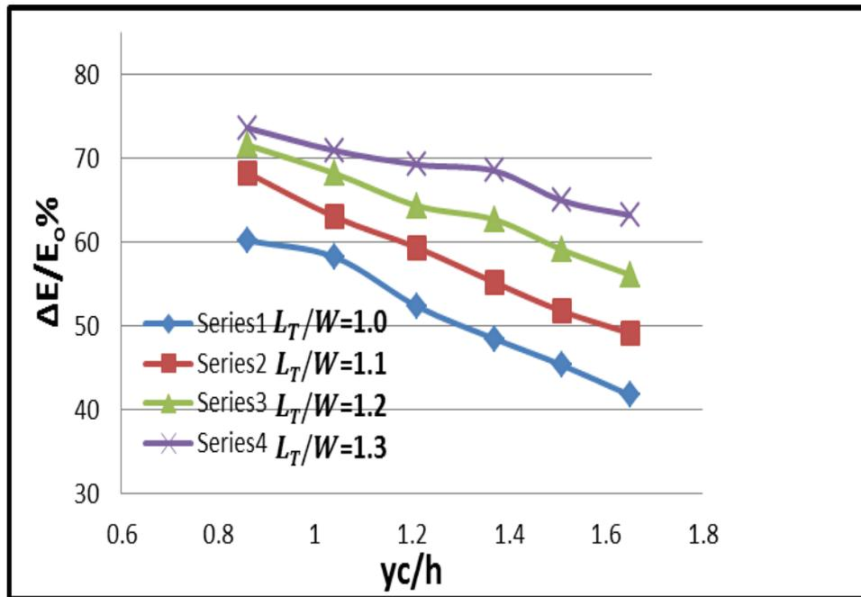
Figure (6) Percentage of energy dissipation with different flow conditions for 35° spillway
