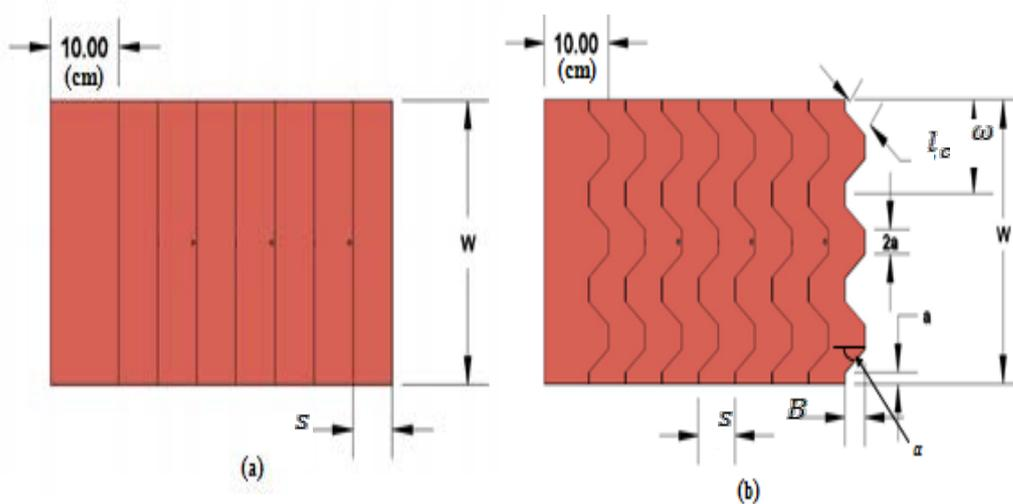
Figure(4) drawing of configuration (a) Traditional shape (b) Labyrinth shape
