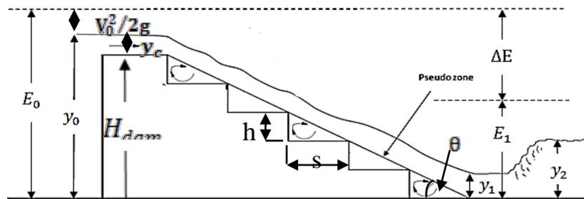
Figure(2) Typical scheme of a stepped spillway
