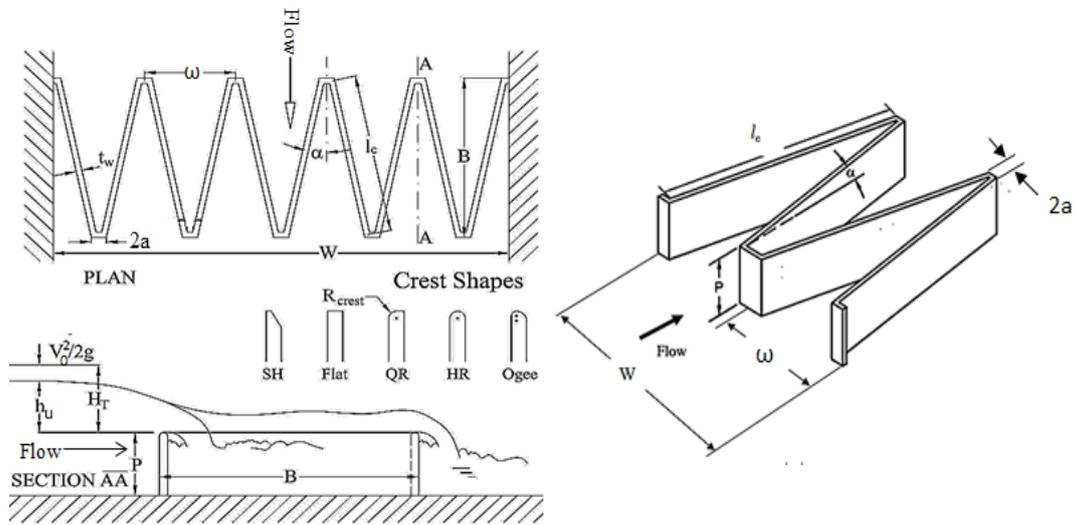
Figure (3) labyrinth weir with related design parameter (Crookston, 2010)
