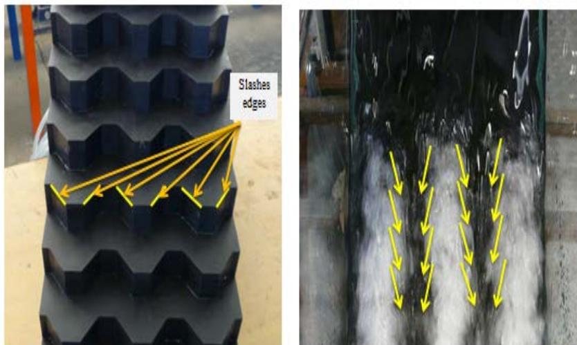
Figure (7) The flow interference over transverse sides of the steps slashes edges
