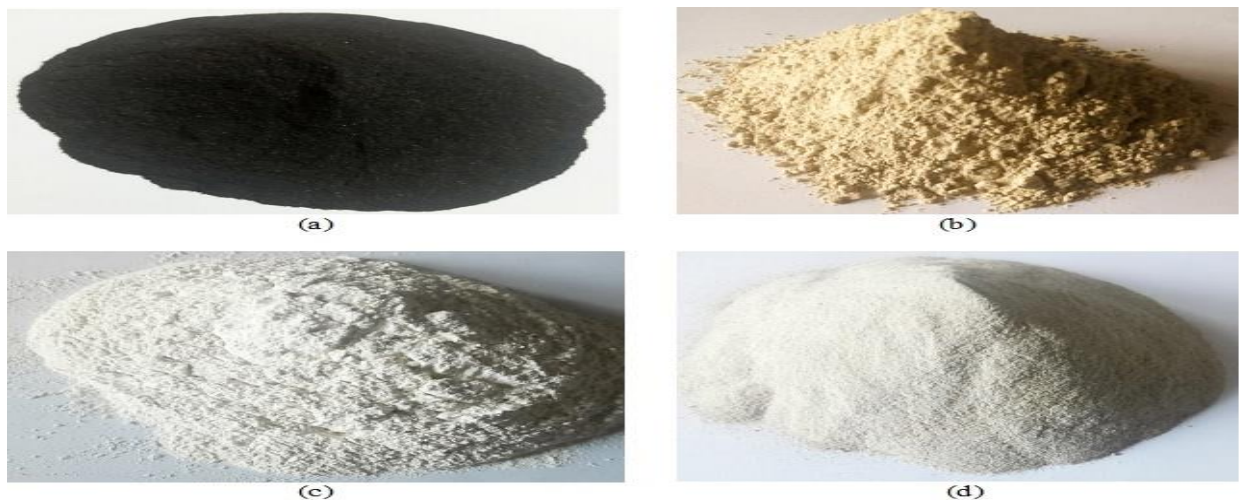
Fig. 1. Photographs of input materials (a) 105 \mu\text{m} iron millscale particles, (b) 53 \mu\text{m} bentonite clay particles, (c) 80 \mu\text{m} magnesia particles, (d) 50 \mu\text{m} silica sand particles.
