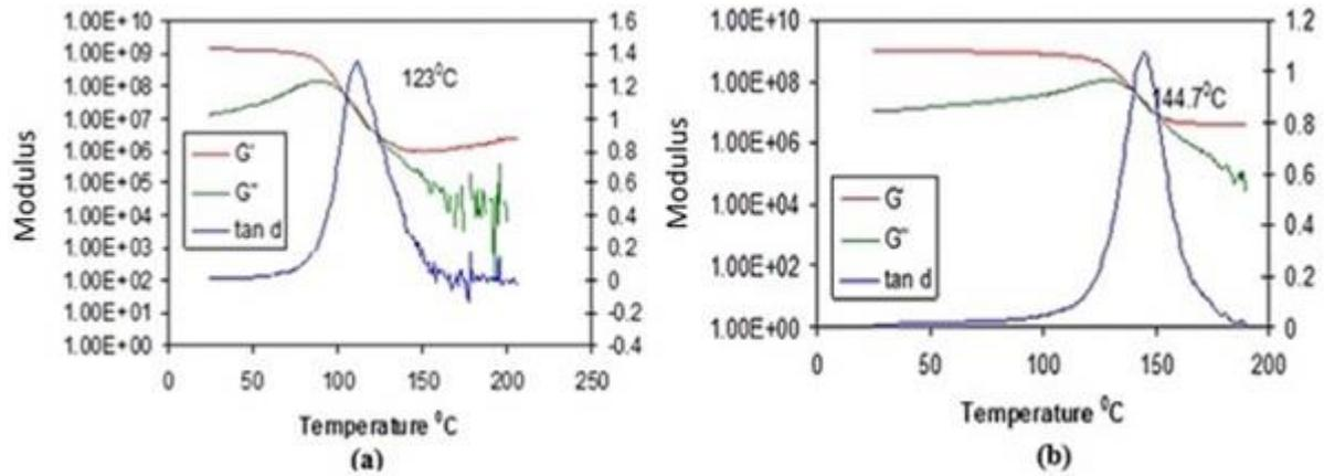
**Fig. 7. Relationship between storage modulus, loss modulus, loss tangent and temperature for the samples (a) Charcoal reinforced (b) Crab shell reinforced.**
