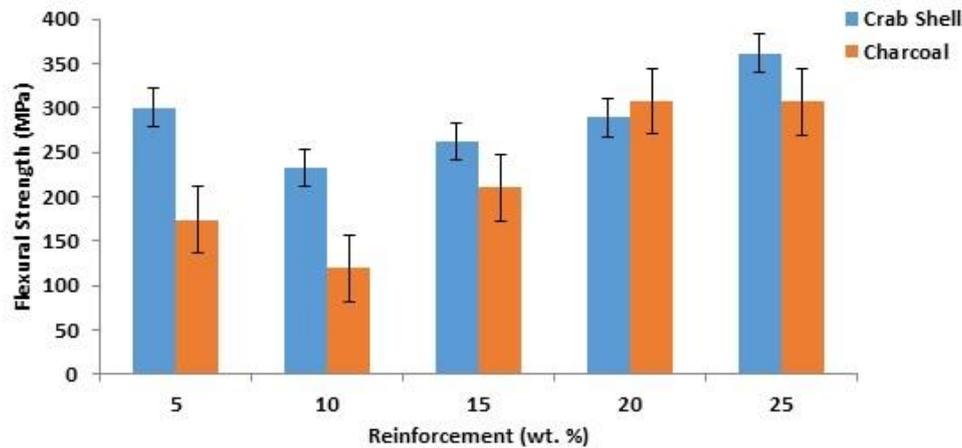
**Fig. 3. Flexural strength of polyester matrix composites with different crab shell and charcoal content.**
