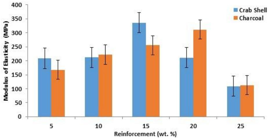
**Fig. 6. Modulus of elasticity of polyester matrix composites with different crab shell and charcoal content.**
