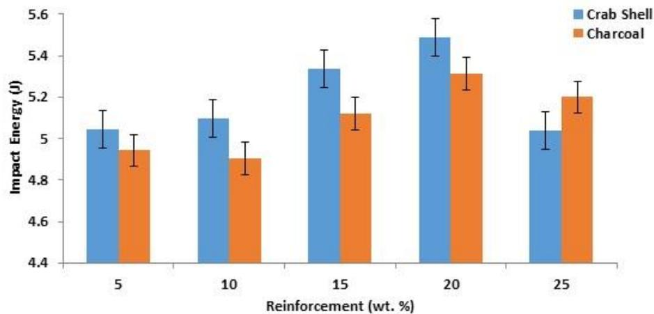
**Fig. 4. Impact energy of polyester matrix composites with different crab shell and charcoal content.**
