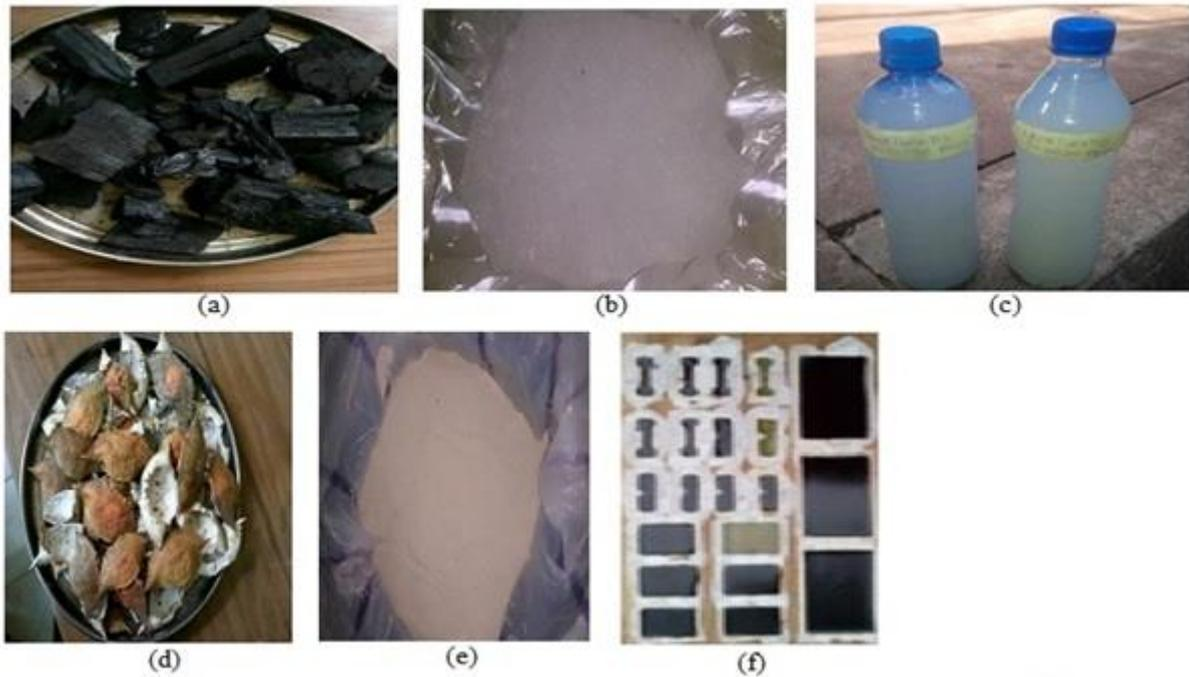
**Fig. 1. Details of the materials (a) Charcoals (b) Grinded charcoal with particle size 150 µm (c) Polyester resin in plastic bottles (d) Crab shell (e) Grinded crab shell with particle size 150 µm (f) Different composite samples in a wooden mould.**
