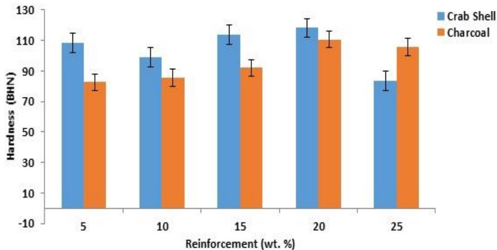
**Fig. 5. Hardness of polyester matrix composites with different crab shell and charcoal content.**
