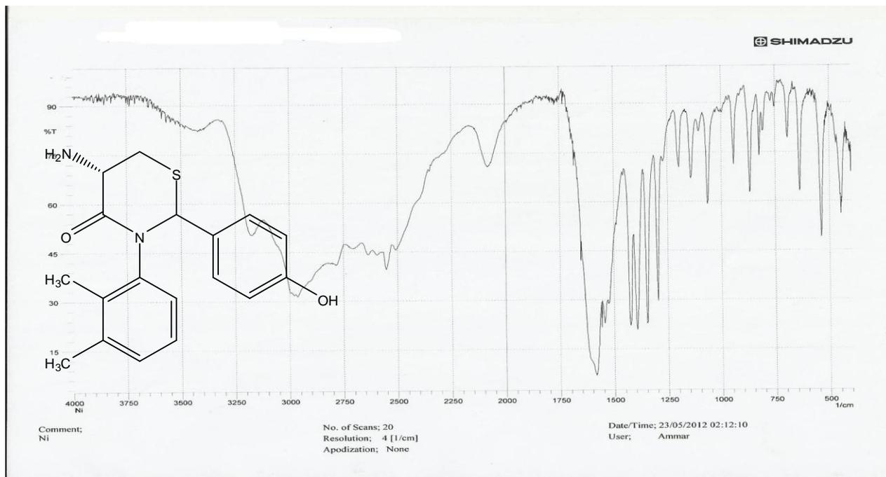
Fig (3-7) show the FTIR spectrum of compound 7 (5S)-5-amino-3-(2,3-dimethylphenyl)-2-(4-hydroxyphenyl)-1,3-thiazinan-4-one
