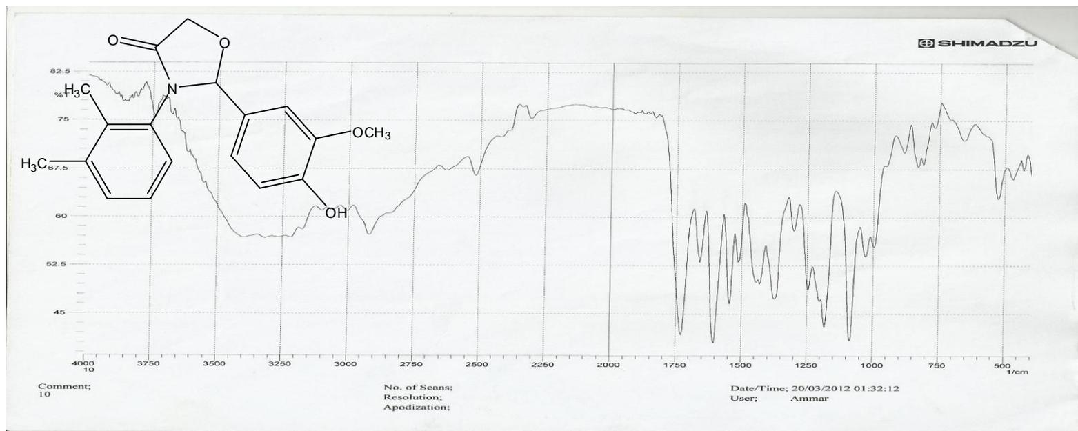
Fig (3-4) show the FTIR spectrum of compound 4 3-(2,3-dimethylphenyl)-2-(4-hydroxy-3-methoxyphenyl)oxazolidin-4-one
