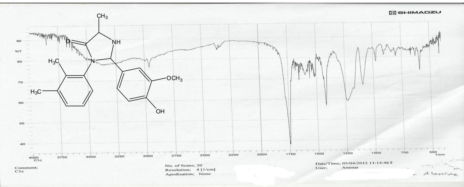
Fig (3-6) show the FTIR spectrum of compound 6 3-(2,3-dimethylphenyl)-2-(4-hydroxy-3-methoxyphenyl)-5-methylimidazolidin-4-one
