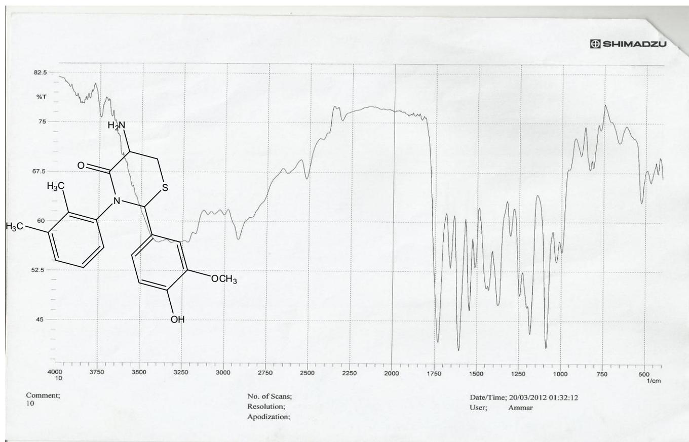
Fig (3-8) show the FTIR spectrum of compound 8 5-amino-3-(2,3-dimethylphenyl)-2-(4-hydroxy-3-methoxyphenyl)-1,3-thiazinan-4-one
