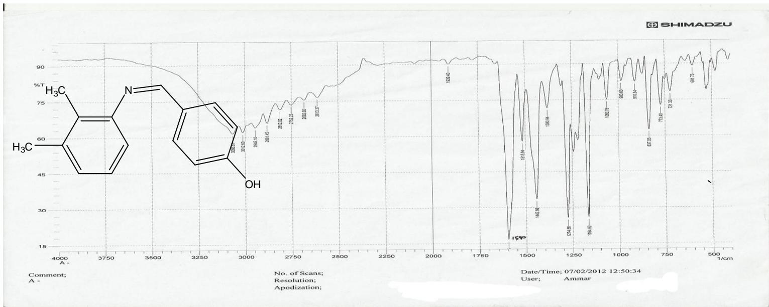
Fig.(3-1) FTIR spectrum of compound 1 (Z)-4-((2,3-dimethylphenylimino)methyl)phenol
