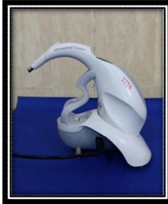
Fig (4) : Spectrophotometer VITA Easyshade Compact.
