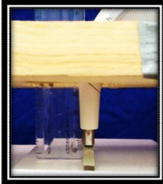
Fig (5) : The tip of VITA Easyshade Compact was perpendicular and in contact with arch wires surface.
