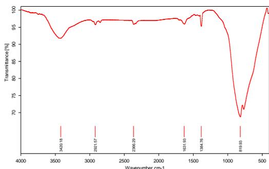
**Figure 12:** FTIR spectrum of WO<sub>3</sub> nanostructures.
