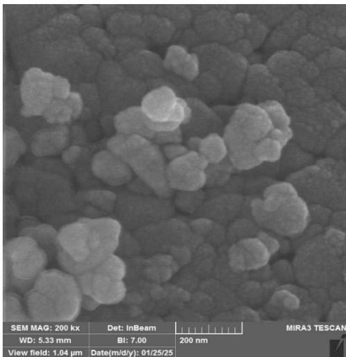
**Figure 10:** FESEM images of green-synthesized WO<sub>3</sub> nanostructures at magnification of (200 nm).
