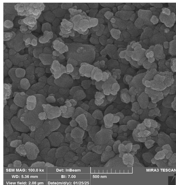
**Figure 9:** FESEM images of green-synthesized  $\text{WO}_3$  nanostructures at magnification of (500 nm).
