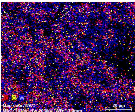
**Figure 6:** EDX elemental mapping of  $WO_3$  nanostructures showing spatial distribution of C, O, and W elements.
