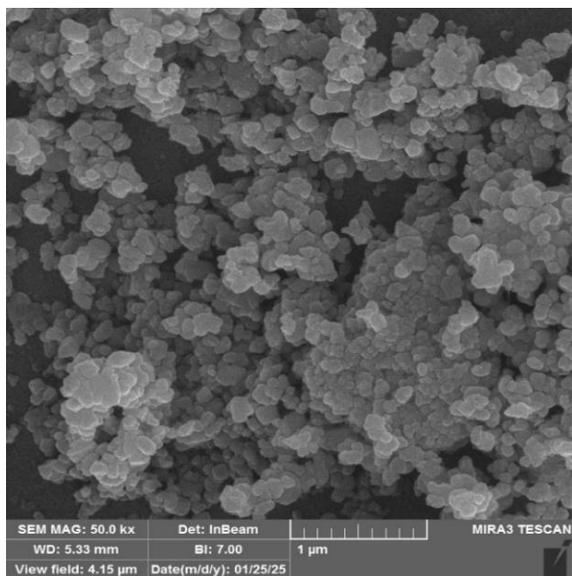
**Figure 7:** FESEM images of green-synthesized  $\text{WO}_3$  nanostructures at magnification of (1  $\mu\text{m}$ ).
