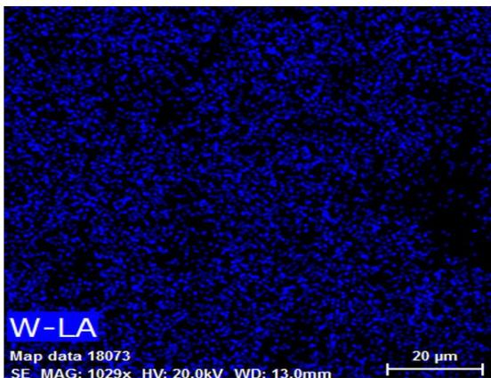
**Figure 5:** EDX elemental mapping of  $WO_3$  nanostructures showing spatial distribution of W element.
