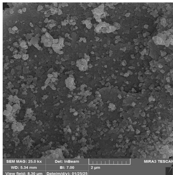
**Figure 8:** FESEM images of green-synthesized  $\text{WO}_3$  nanostructures at magnification of (2  $\mu\text{m}$ ).
