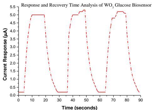
**Figure 13:** Response and recovery time analysis of WO<sub>3</sub> Glucose biosensor.
