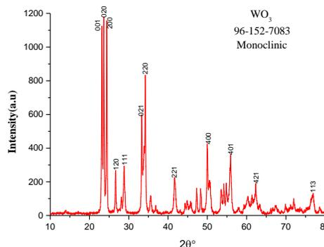
**Figure 1:** XRD pattern of monoclinic WO<sub>3</sub> nanostructures.
