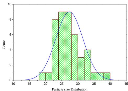
**Figure 11:** Histogram showing particle size distribution of WO<sub>3</sub> nanostructures with a mean diameter of 27.376 nm and a normal distribution curve (blue line).
