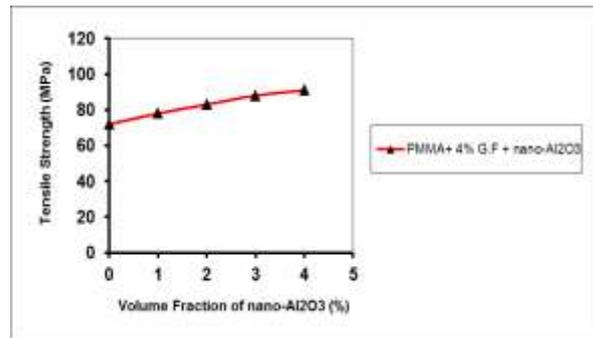
**Figure 6: Tensile Strength of PMMA Hybrid Laminated Composite as Function of (Nano-Al<sub>2</sub>O<sub>3</sub>) Particles (Vol. %) in Composite.**
