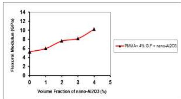
Figure 11: Flexural Modulus of PMMA Hybrid Laminated Composite as Function of (Nano-Al<sub>2</sub>O<sub>3</sub>) Particles (Vol. %) in Composite.
