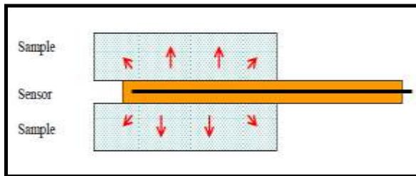
Figure 15: Hot Disk Sensor Operation.
