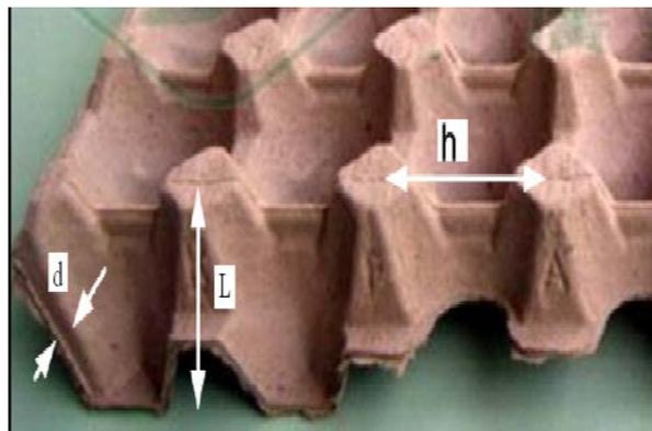
Figure (2) Appearance of the pyramidal base form
