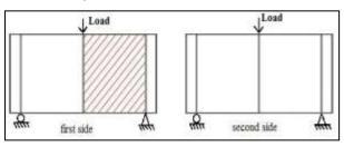
Figure 5: Strengthening technique used for girder (T2-1)
