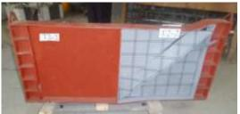
C) Plate Girder (T2-2) after Testing
