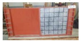
D) Plate Girder (T2-3) after Testing Figure 12: Tested Plate Girders after Failure after testing
