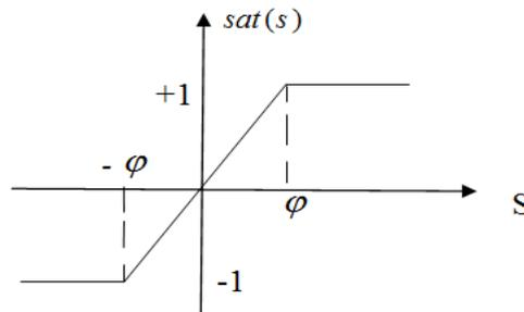
**Figure (3): The sat(s) function.**
