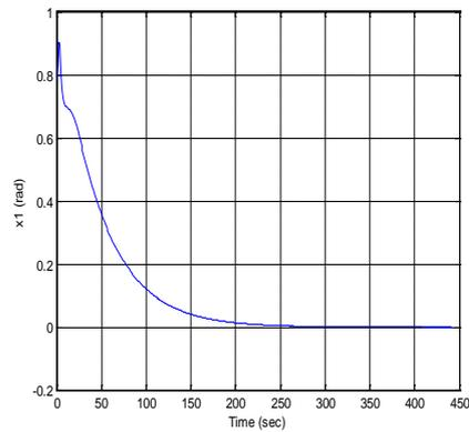
**Figure (8): The plot of the output  $\theta$  with time. Figure (9): The plot of the error  $x_1$  with time.**
