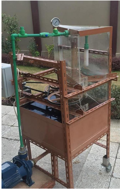
Fig. 1. Photograph of jet erosion tester.
