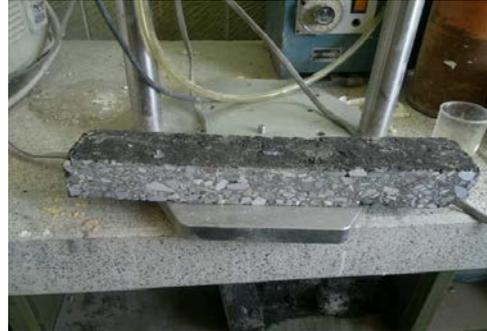
Figure (8): Beam fatigue test (specimen after test)
