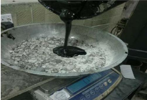
Figure (5): Mixing of asphalt binder and aggregate
