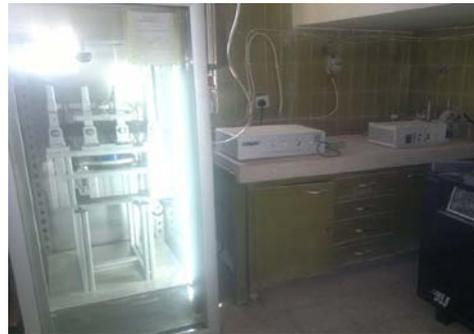
Figure (9): Beam fatigue Test: testing device
