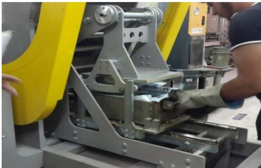
Figure (6): Slab preparation in Roller Compactor machine
