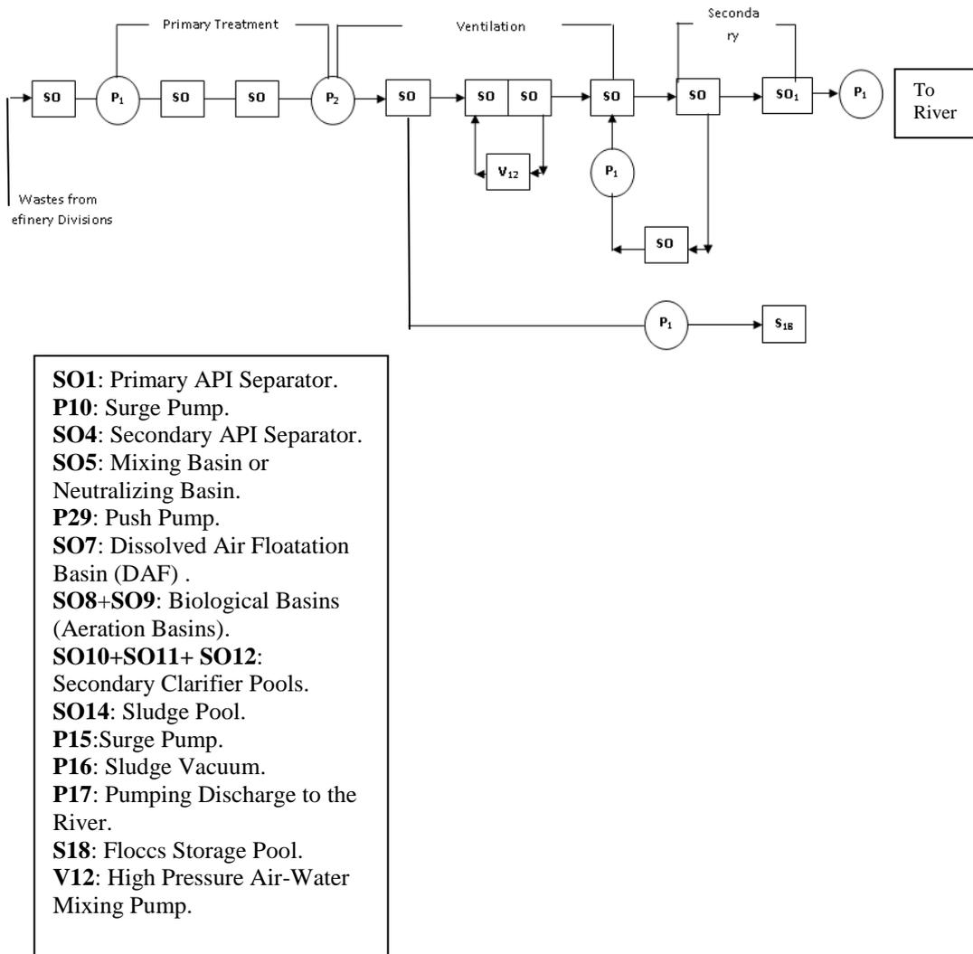
**Figure. (1) Sketch represents main components of wastes treatment unit for Al-Dura refinery (Iraqi ministry of oil/Midland refineries co. / AL-Dura refinery).**
