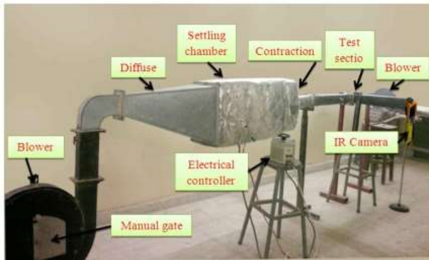
Figure (2) Photograph of the test rig.
