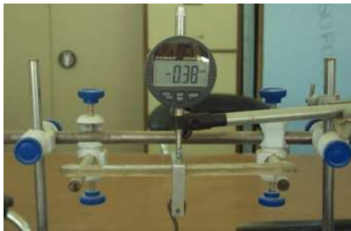
Figure (1)3-Point Bending Tests Device With Composite Specimen.
