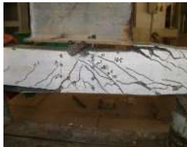
Figure (25) cracks pattern of beam (B7).
