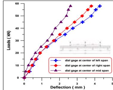
Figure (14) Load – Deflection curve for beam (B1).
