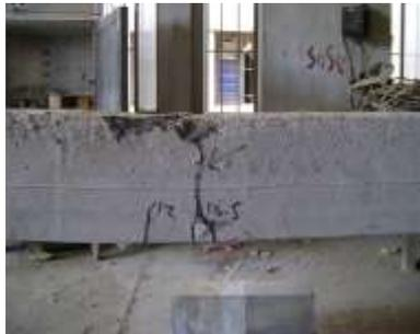
Figure (13) cracks pattern of beam (B1).
