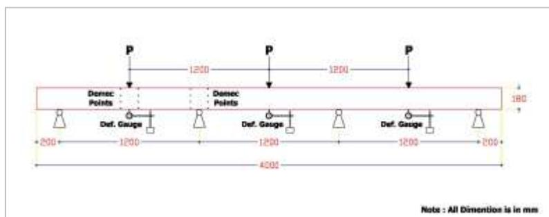
Figure (12) The locations adopted for measuring deflections and longitudinal strains
