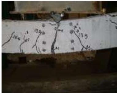
Figure (15) cracks pattern of beam (B2).
