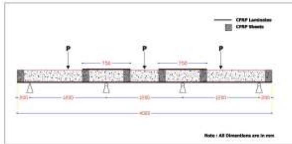
Figure (9) Schematic of specimen B7 with bonded CFRP strips.
