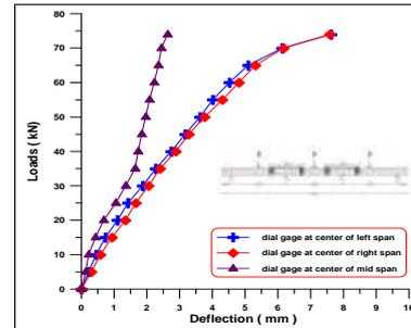
Figure (16) Load – Deflection curve for beam (B2).
