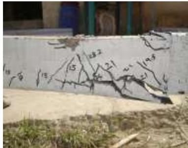
Figure (23) cracks pattern of beam (B6).
