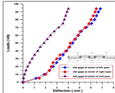
Figure (24) Load – Deflection curve for beam (B6).
