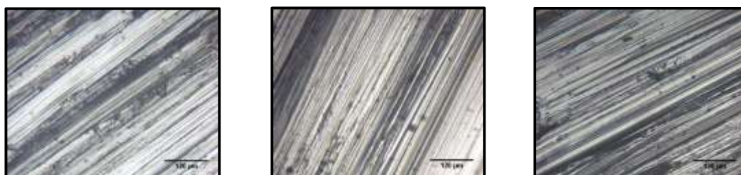
Figure7: The microstructure of Al-Mg-Si alloy after wear test (a) 5N applied load of (Ex.No.2), (b) 10N applied load (Ex.No.5), (c) 15N applied load (Ex.No.8)
