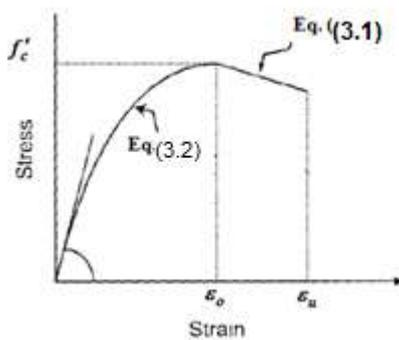
Figure (3.2): Stress-strain relationship of concrete in compression [14].
