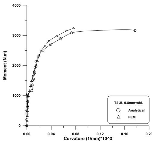
**Figure (4.12): Numerical and analytical moment-midspan curvature curves of T-beam T2**
