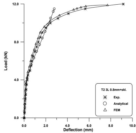
Figure (4.10): Experimental and load-midspan deflection curves of T-beam T2
