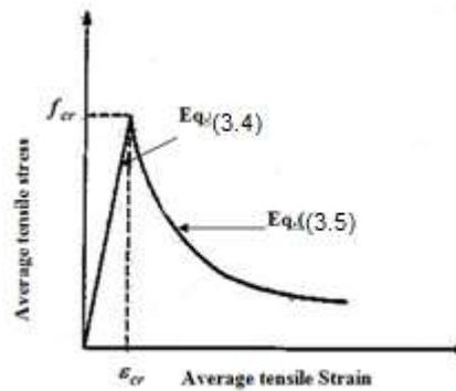
Figure (3.3): Average tensile stress-strain curve for concrete [15].
