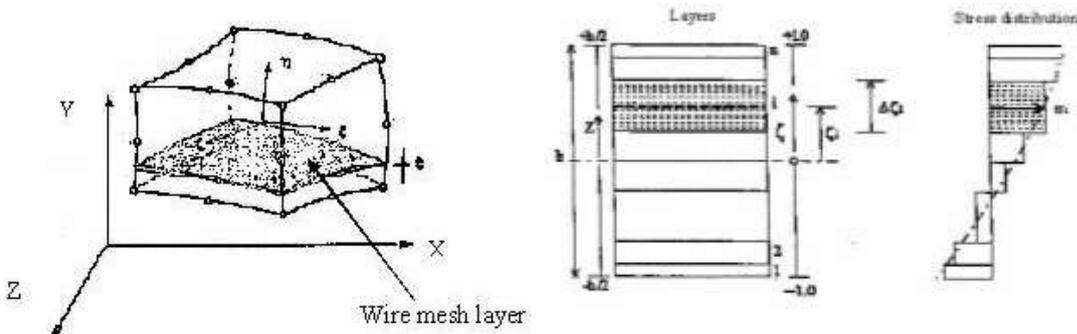
Figure (2.2): Three-dimensional solid element with layered system.
