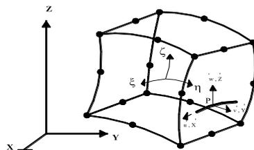
**Figure (2.4): Embedded representation of reinforcement.****Embedded Bar Reinforcement Idealization**
