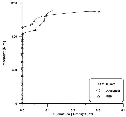
Figure (4.12): Numerical and analytical moment-midspan curvature curves of response T-beam T1
