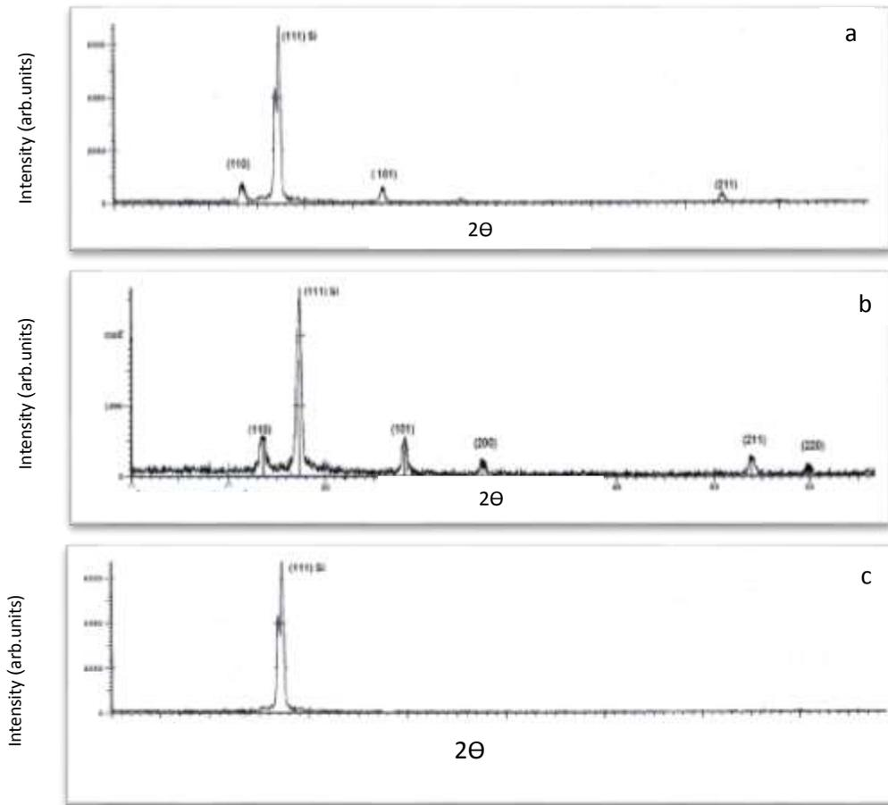
**Figure (2) XRD patterns of SnO<sub>2</sub> films grown on Si at various oxygen pressures a)  $5 \times 10^{-2}$  mbar b)  $5 \times 10^{-1}$  mbar c).**
