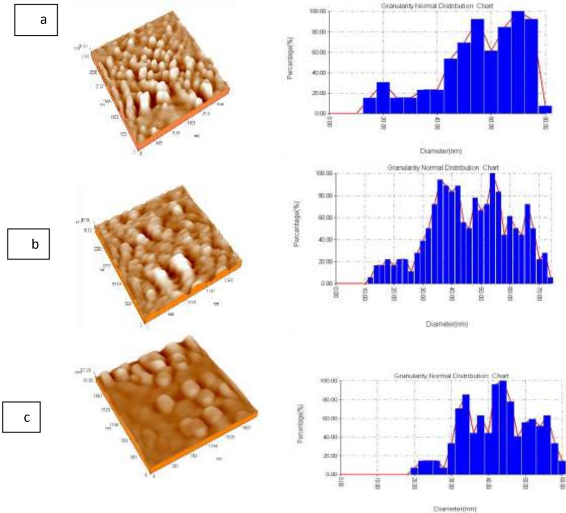
Figure(3)AFM image of theSnO<sub>2</sub>/Si thin films deposited at various oxygen pressure a ) 5\*10<sup>-2</sup> mbar, b) 5\*10<sup>-1</sup> mbar and c) 10 mbar at substrate temperature 300 °C and 1.2 J/cm<sup>2</sup> laser fluence energy
