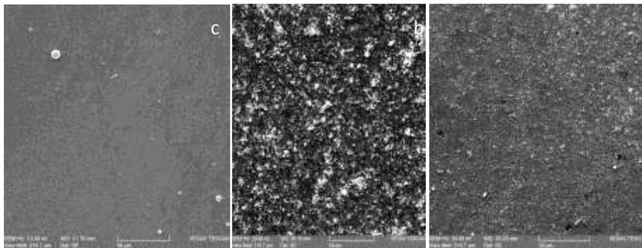
Figure (4) SEM image of the SnO<sub>2</sub>/Si thin films deposited at various oxygen pressure a)  $5 \times 10^{-2}$  mbar, b)  $5 \times 10^{-1}$  mbar and c) 10 mbar at substrate temperature 300 °C and 1.2 J/cm<sup>2</sup> laser fluence energy
