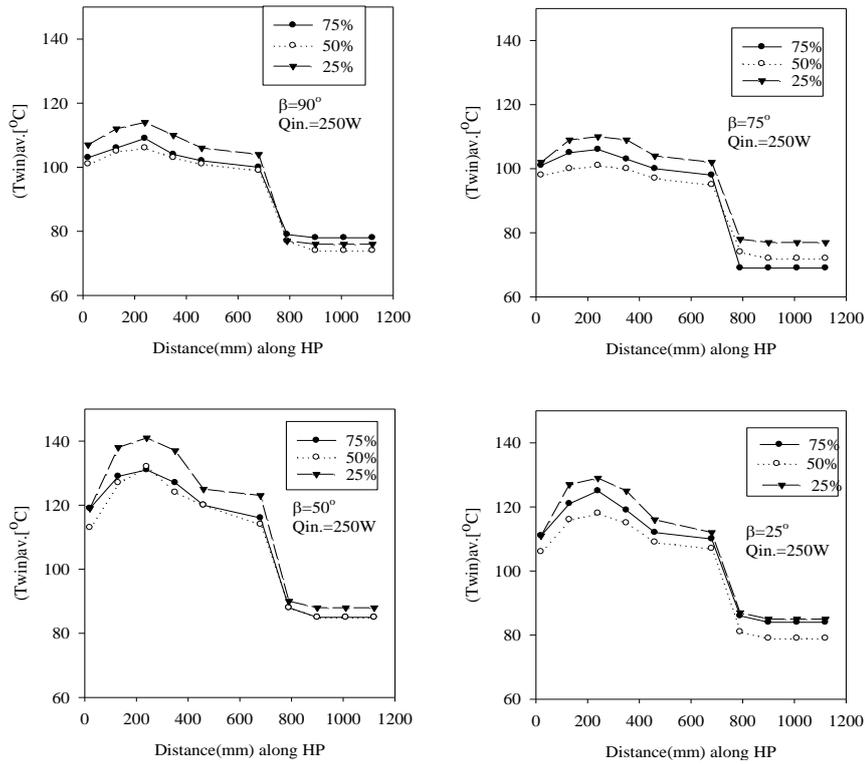
Figure(3):Variation of average wall temperature along the HP at different heptane filling ratios and orientations for a given power input.
