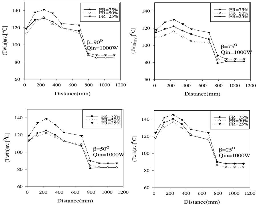
Figure(4) Variation of average wall temperature along the HP at different filling ratios and orientations at a given power input.
