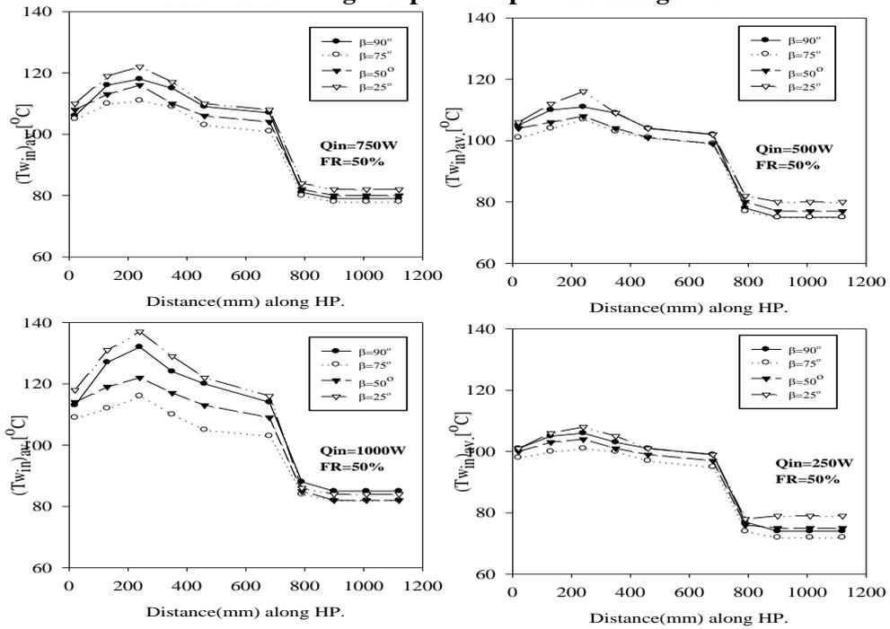
Figure(8) Variation of average wall temperature along HP with different orientations at a given power input.
