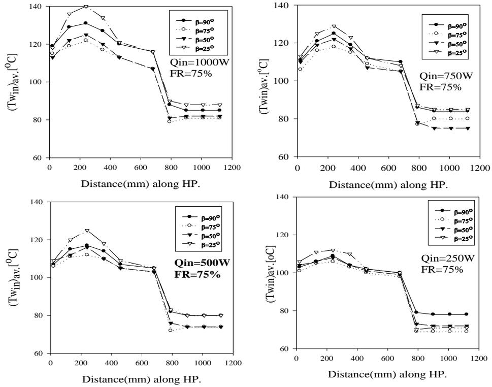
Figure(7) Variation of average wall temperature along HP with different orientations at a given power input and filling ratio.
