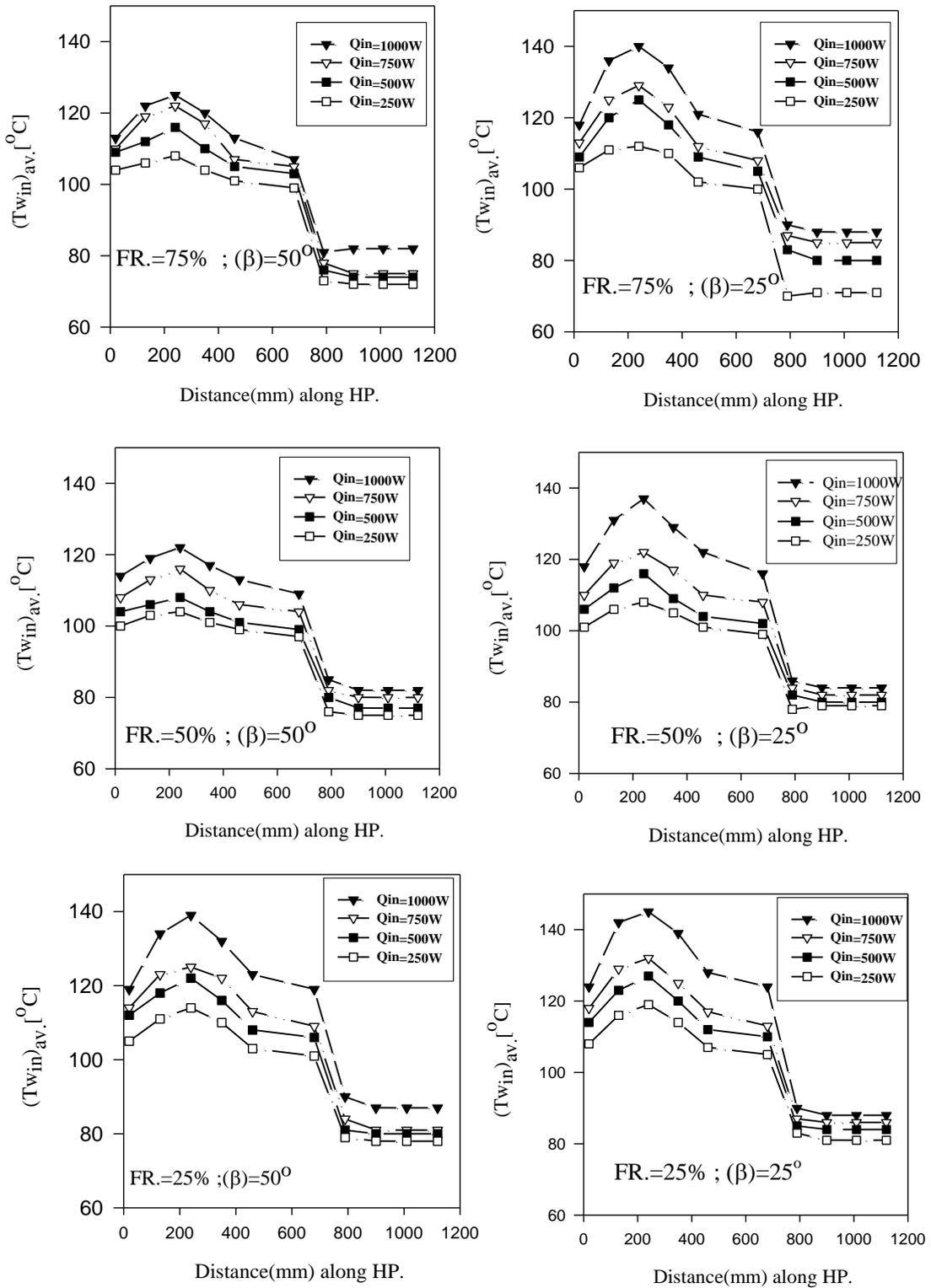
Figure (6) Variation of average wall temperature along the HP with different powers and filling ratios at a given orientation.
