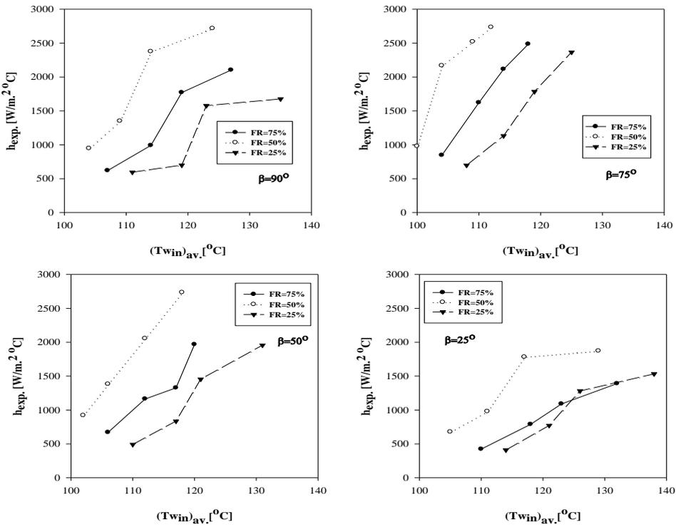
Figure(10) Heat transfer coefficient vs. average wall temperature of evaporator at a given power input different filling ratios and a given inclination angle.
