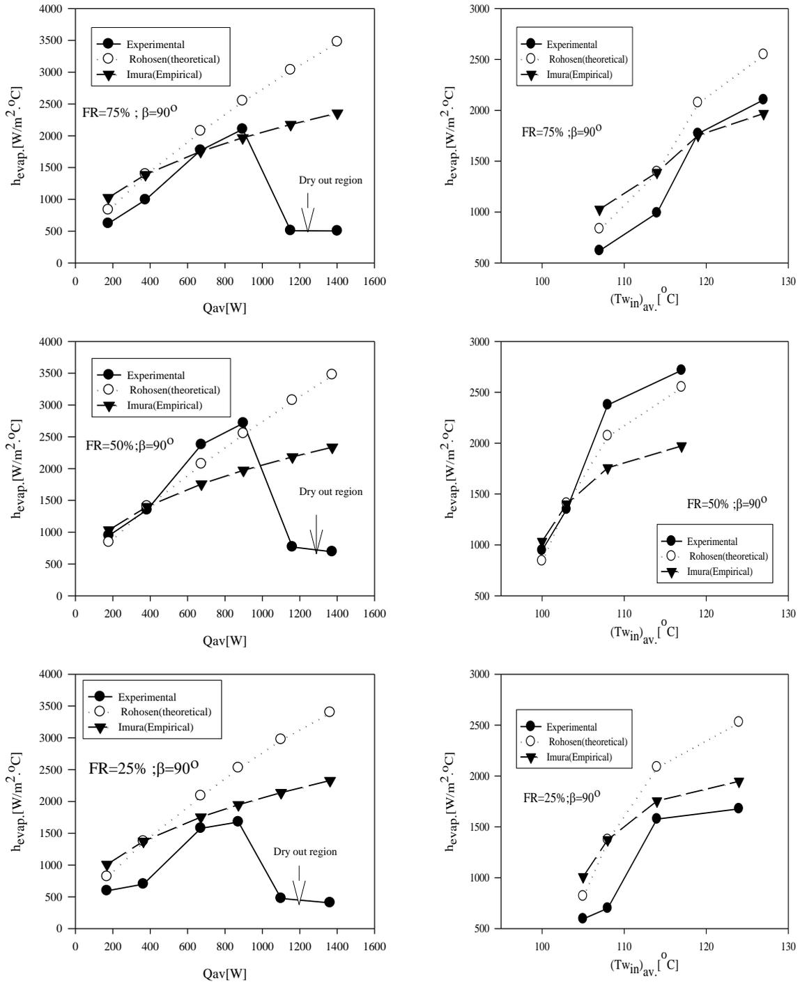
Figure(11) Heat transfer coefficient vs. average heat input for experimental, theoretical and empirical correlations at inclination angle  $90^\circ$  and diff. FR.
