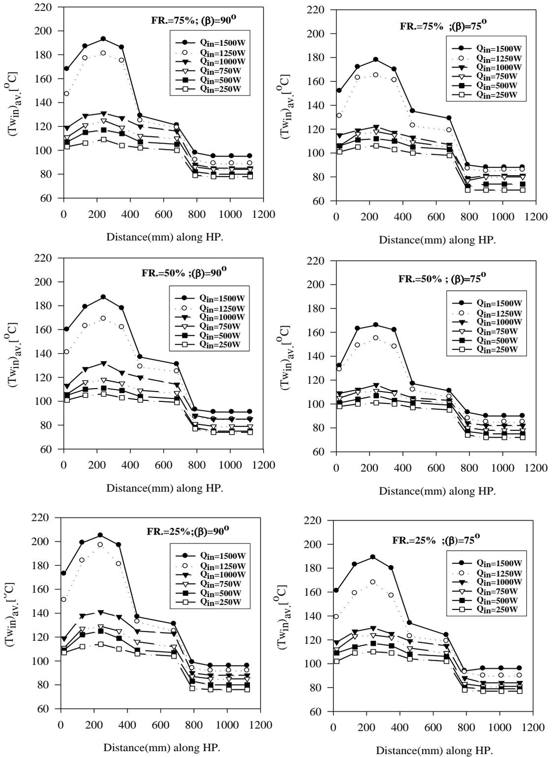
Figure(5) Variation of average wall temperature along the HP at different heating loads and filling ratios for a given orientation.
