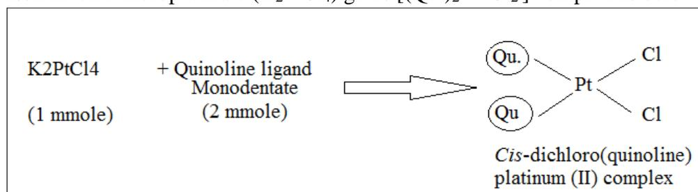
**Figure(2): Synthesis of Cis- dichloro(quinoline)2 plsatinum (II) complex.**
