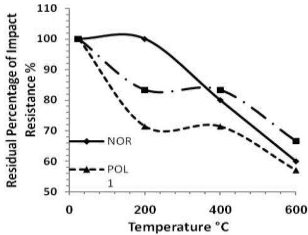
Figure (17) Residual Percentage of Impact Resistance for mixes at each level of temperature.
