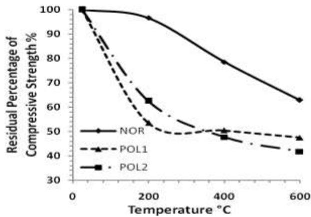
Figure (6) Residual Percentage of Compressive Strength for mixes at each level of temperature.
