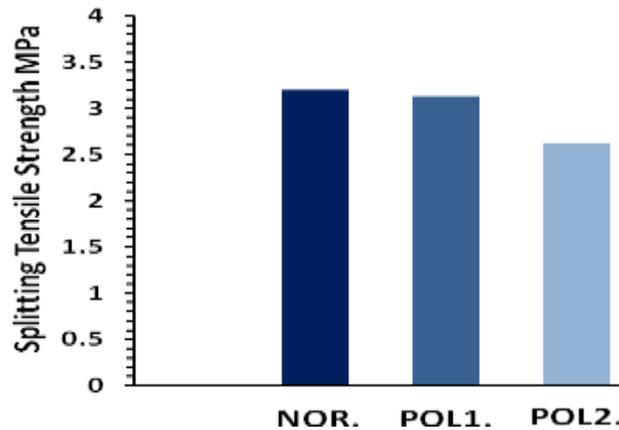
Figure (7) Splitting Tensile Strength of Concrete Mixes in Lab Temperature.
