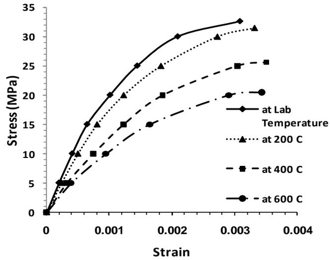
Figure (10) Stress-Strain Relation neither for Normal Concrete NOR at each level of temperature.
