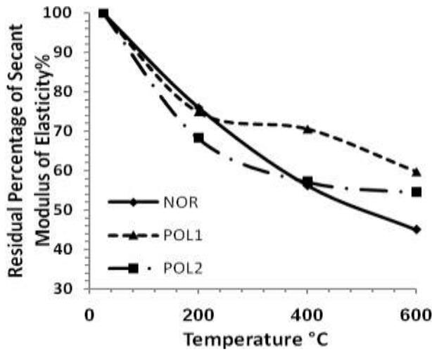
Figure (13) Residual Percentage of Secant Modulus of Elasticity for mixes at each level of temperature.
