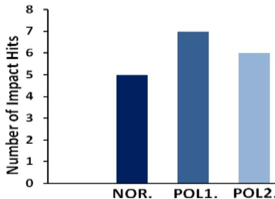
**Figure (14) Number of Impact Blow up for Mixes of Concrete at Lab Temperature.**
