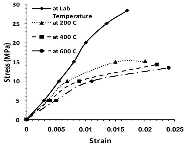
Figure (11) Stress-Strain Relation for Polymerized Concrete POL1 at each level of temperature.
