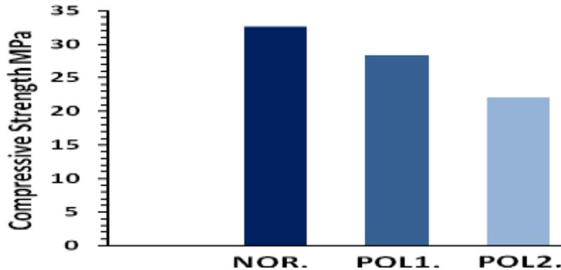
Figure (5) Compressive Strength of Concrete mixes in Lab Temperature
