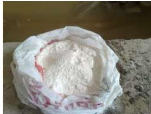
**Figure (1) Sodium carboxy-methyl cellulose E466 (CMC).**
