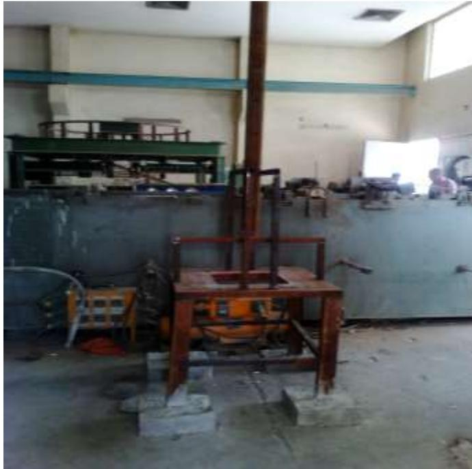
**Figure (4) Frame for Impact Resistance Test.**
