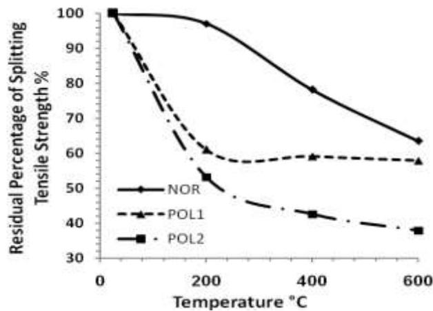
Figure (8) Residual Percentage of Splitting Tensile Strength for mixes at each level of temperature.
