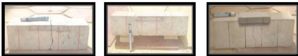
(a) (b) (c) Figure (6) Failure modes of composite section beam, (a) the failure at the centre, (b) the failure at edge of the notch section, and (c) the failure as de- lamination notch section.
