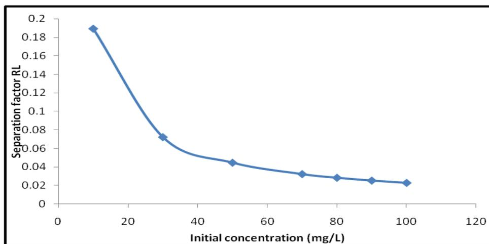
**Figure(9) : Separation factor versus initial (RB5) concentration on to (RHC)**
