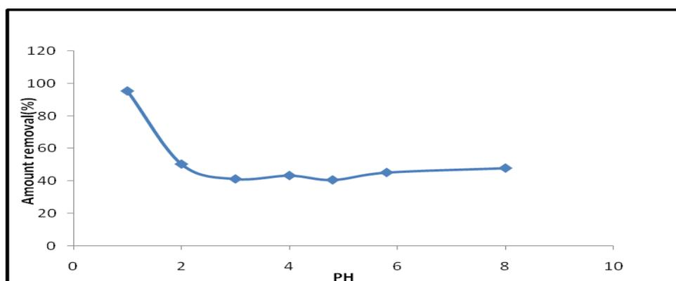
**Figure(6) : Adsorption of (RB5) by (RHC) as a function of solution pH at initial concentration of 50 mg/l and adsorbent dosage of 1.5 g with 300 $\mu$ m particle size**
