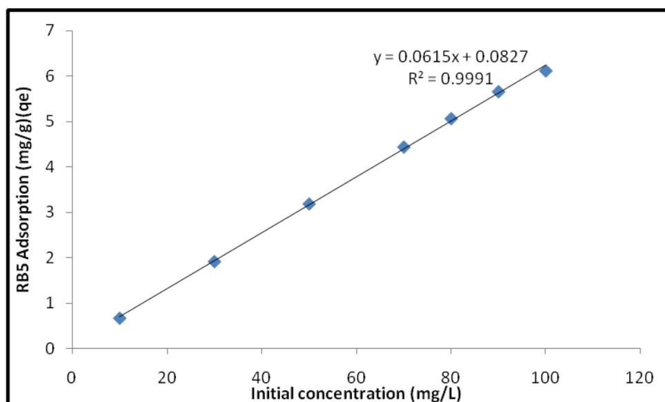
**Figure(7) : Effect of initial concentration on adsorption capacity of (RB5) onto (RHC) (300 $\mu$ m particle size and 1.5gm adsorbent dose)**
