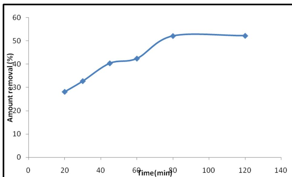
**Figure ( 4 ) : Effect of contact time for adsorption of (RB5) onto (RHC) at initial dye concentration of 50 mg/l, adsorbent dose of 1.5 g and particle size of 420 $\mu$ m**
