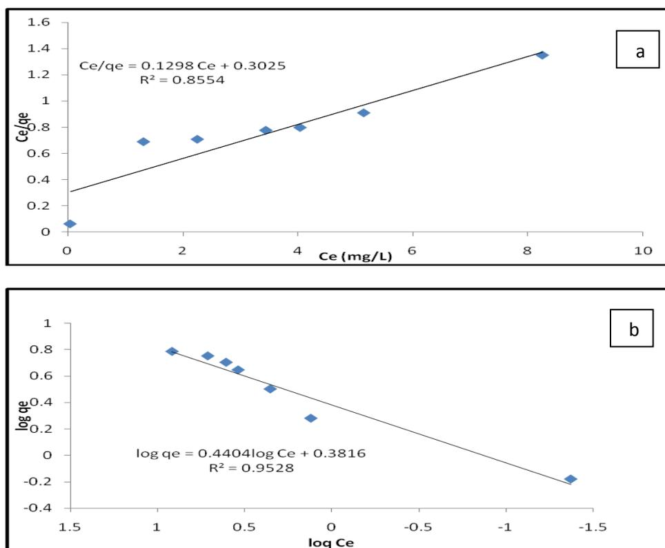
Figure(8): Linearized adsorption isotherm model of (RB5) onto (RHC)
