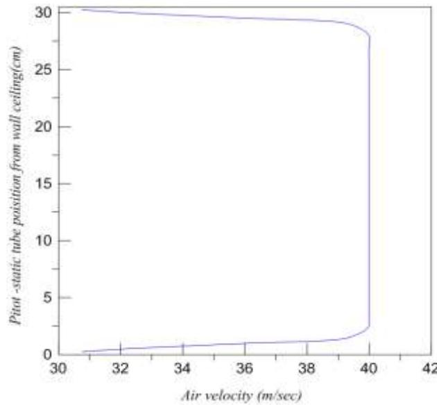
Figure (8) Air velocity distribution in the fan inlet duct.
