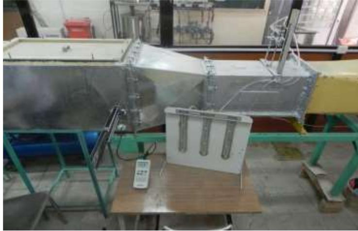
Figure (6) Pitot - static tube with manometer at fan inlet duct.
