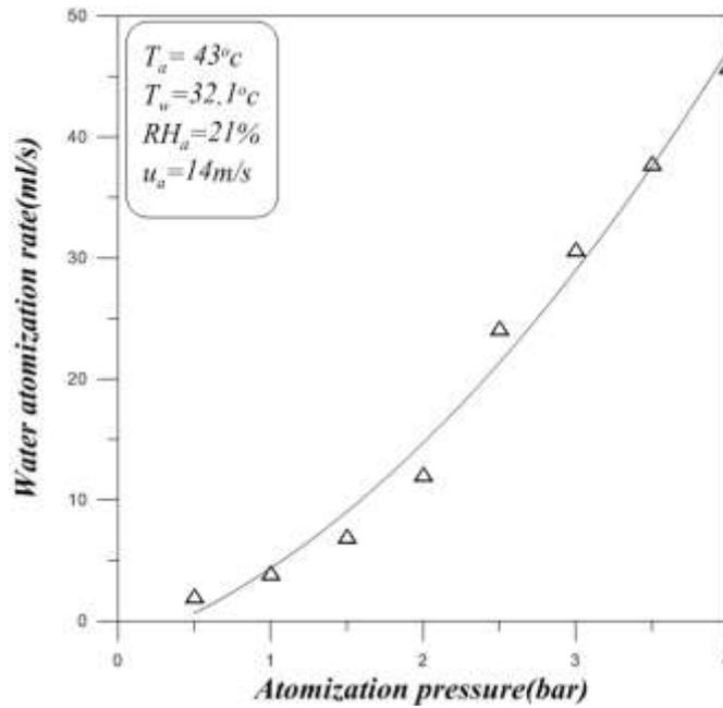
Figure (9) Relation between water atomization rate and atomization pressure.
