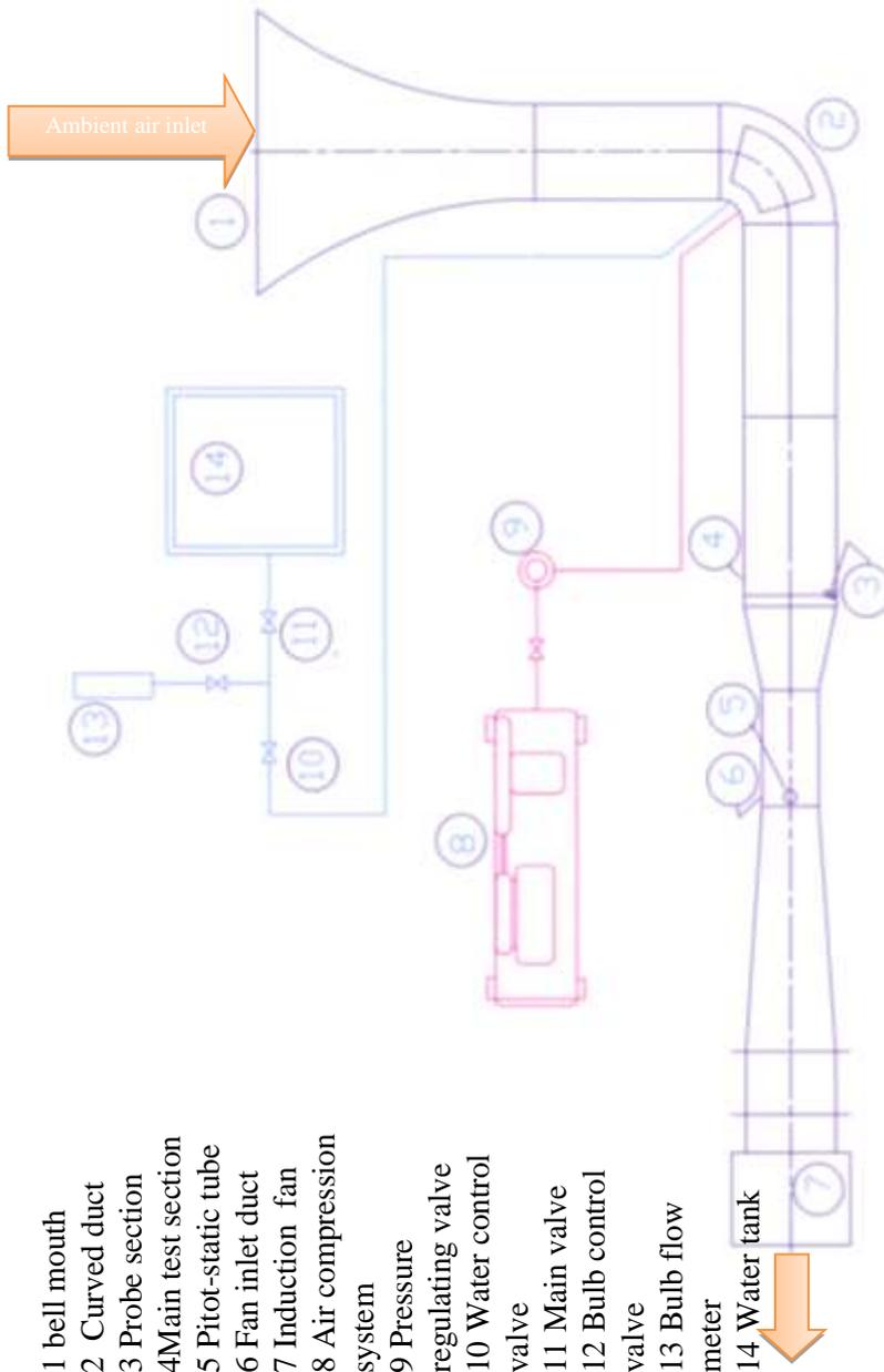
The atomizer used in this work has a diameter of (2.5 mm), and working at a safe pressure of (3.8 bar). The atomizer is used to introduce water in the form of fine droplets. This atomizer slides radially between 5 to 45 cm from the inner wall of the curved duct and it is mounted on a bracket that has the ability to rotate from -90° to +90° to the tangential flow direction by a step of 5° as illustrated in Figure (5).
