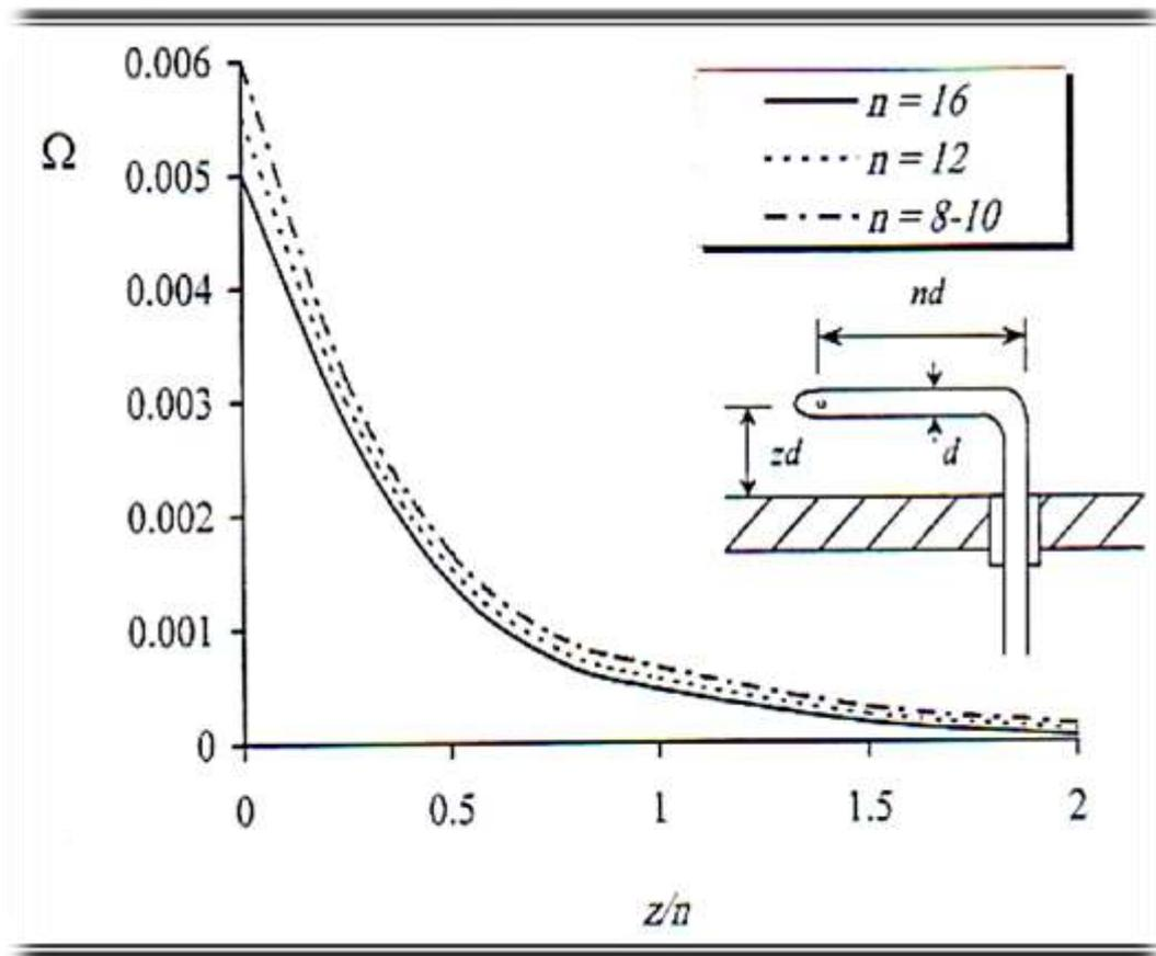
Figure (18) Correction Pitot - static tube.
