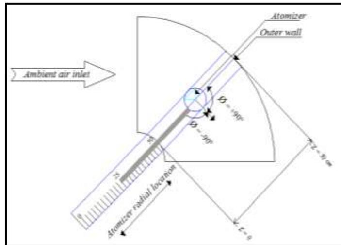
**Figure (5) Details of atomizer movements in the curved duct.**
