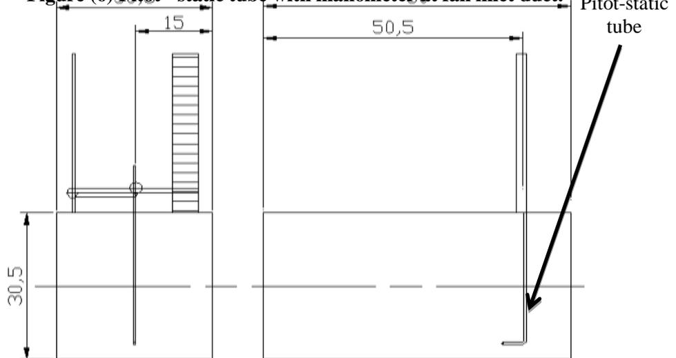
Figure (7).Pitot - static tube.
