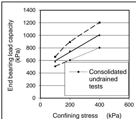
Figure (7) End Bearing Load Capacity Versus Confining pressure for Full Penetrating Sand column-  $a_s=11\%$ .(Heba H.Ali, 2007)
