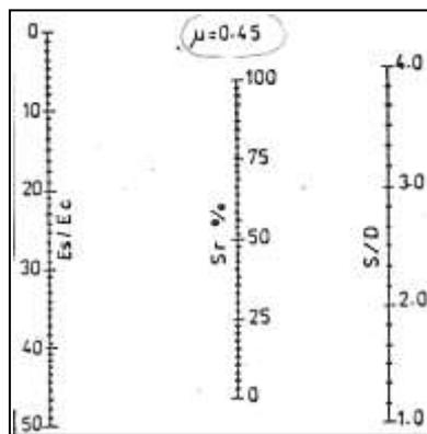
**Figure (2) Nomogram of Relationship Between Es/Ec and Ratio of Settlement for Soil with  $\nu=0.45$ .**
