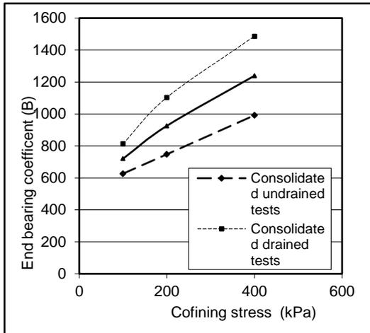
**Figure (9) End Bearing Coefficient Versus Confining Pressure for Full penetration Sand column- as=11%. (Heba H.Ali, 2007)**
