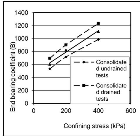
**Figure (10) End Bearing Coefficient Versus Confining Pressure for Full penetration Sand column- as=6%. (Heba H.Ali, 2007)**
