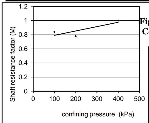
Figure (3) Shaft Resistance Factor (M) Versus Confining Pressure for Clay Media-  $a_s=11\%$ .
