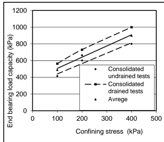
Figure (8) End Bearing Load Capacity Versus Confining pressure for Full Penetrating Sand column-  $a_s=6\%$ . (Heba H.Ali, 2007)
