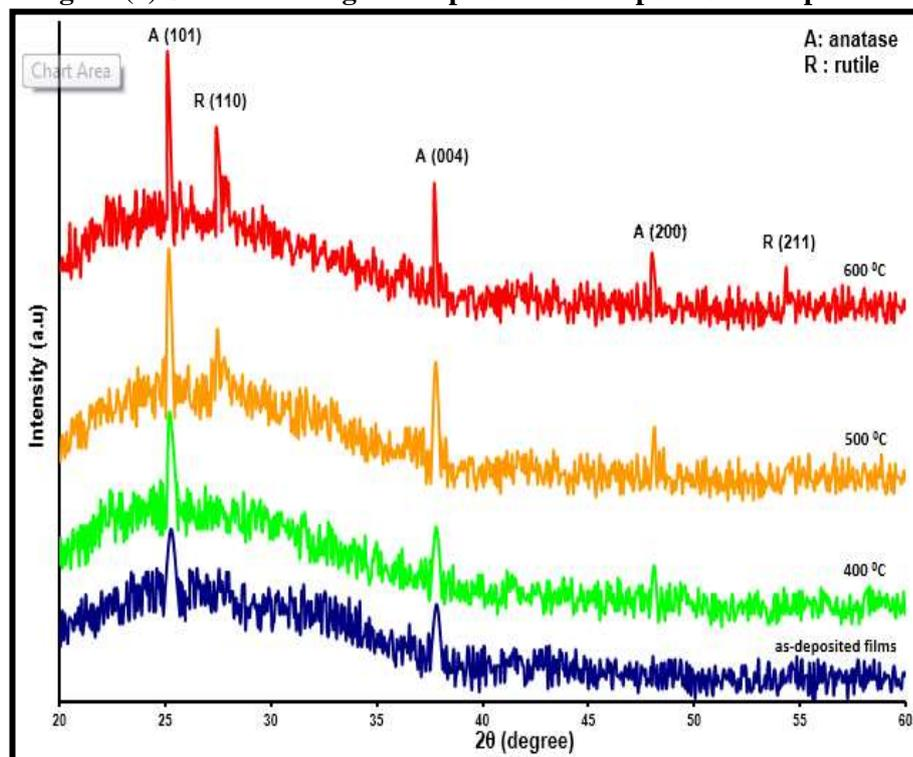
Figure (2) XRD patterns of TiO<sub>2</sub> films deposited at 300 °C temperature and annealed at 400 °C, 500 °C and 600 °C.
