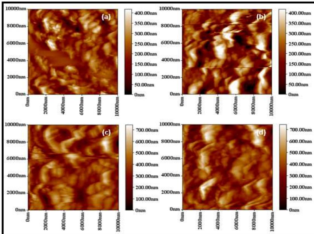
Figure (3) AFM images of TiO<sub>2</sub> films deposited at 300 °C temperature and annealed at different temperatures: (a) As-deposited, (b) 400 °C, (c) 500 °C and (d) 600 °C.
