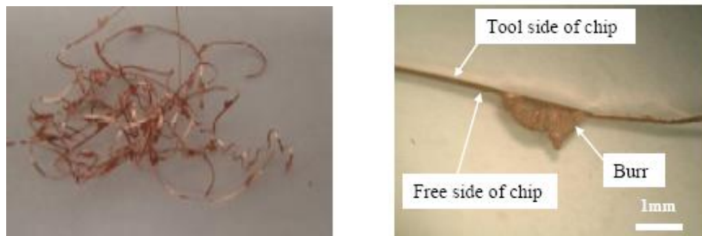
Figure 9 - Micrographs of Cu-Ni chips produced in machining with WC tool.
